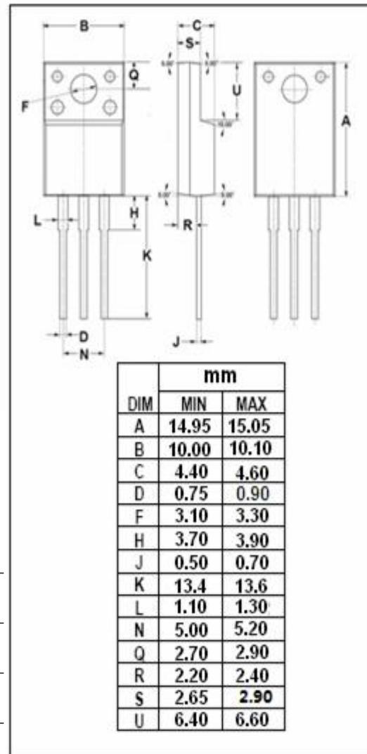
**isc N-Channel MOSFET Transistor**
