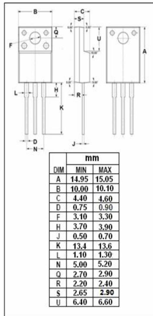
**Isc N-Channel MOSFET Transistor****IPA65R110CFD****ELECTRICAL CHARACTERISTICS** $T_c=25^\circ\text{C}$  unless otherwise specified
