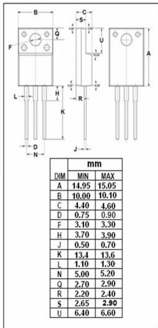
**Isc N-Channel MOSFET Transistor****IPA60R600P7****ELECTRICAL CHARACTERISTICS** $T_c=25^\circ\text{C}$  unless otherwise specified
