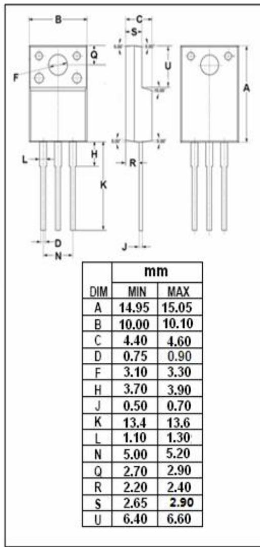
**Isc N-Channel MOSFET Transistor****IPA60R280C6****ELECTRICAL CHARACTERISTICS** $T_c=25^\circ\text{C}$  unless otherwise specified
