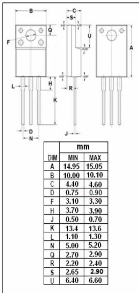
**Isc N-Channel MOSFET Transistor****IPA60R190P6****• ELECTRICAL CHARACTERISTICS****T<sub>c</sub>=25°C unless otherwise specified**
