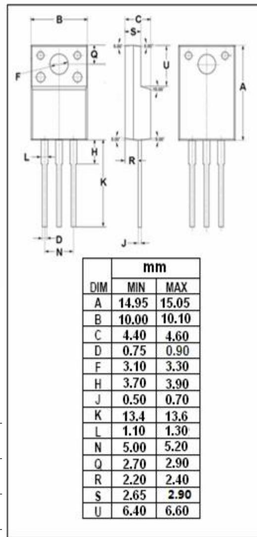
**isc N-Channel MOSFET Transistor****IPA60R160C6****ELECTRICAL CHARACTERISTICS** $T_c=25^\circ\text{C}$  unless otherwise specified
