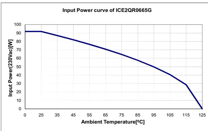
Figure 13 Input Power curve  $V_{in}=230\text{Vac}; P_{in}=f(T_a)$
