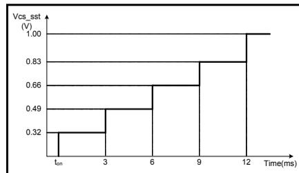
Figure 4 Maximum current sense voltage during softstart
