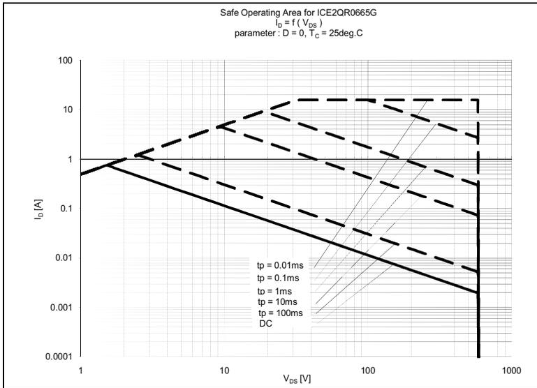
Figure 9 Safe Operating Area(SOA) curve for ICE2QR0665G
