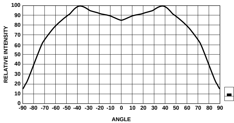
Figure 6. Relative intensity vs. angle for HSMx-C120.
