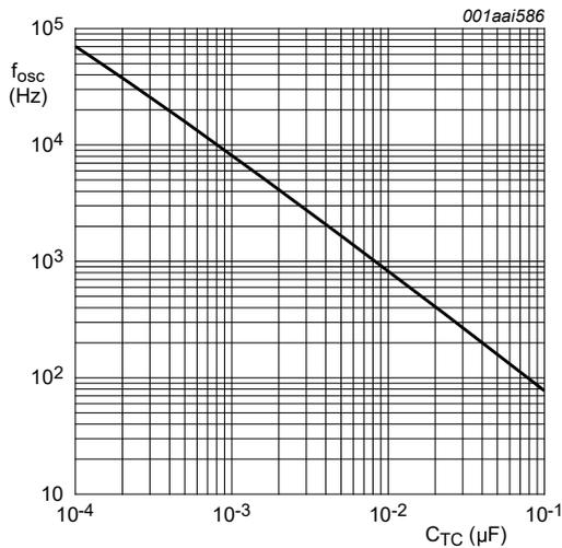
a.  $C_{TC}$  curve at  $R_{TC} = 56$  k $\Omega$ ;  $R_S = 120$  k $\Omega$ .
