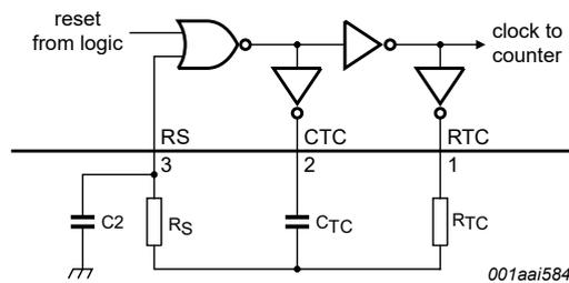
Typical formula for oscillator frequency:  $f_{osc} = \frac{1}{2.3 \times R_{TC} \times C_{TC}}$
