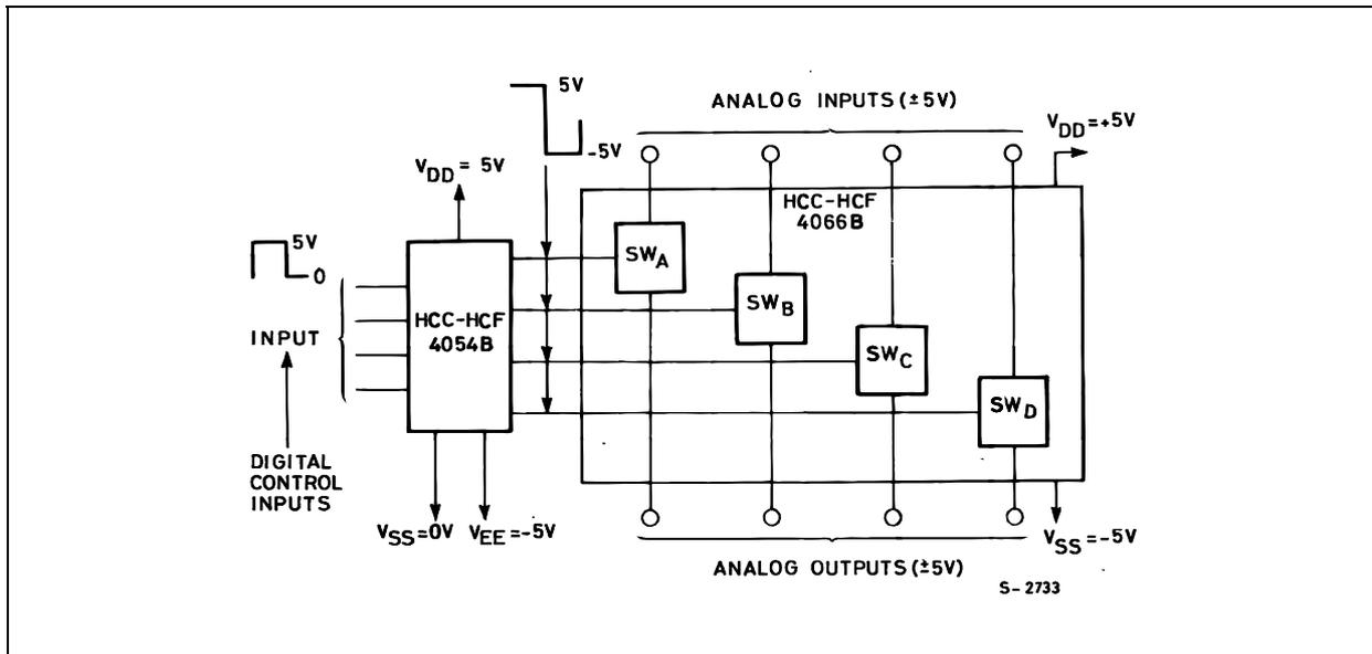
TYPICAL APPLICATIONS (4-CHANNEL PAM MULTIPLEXER SYSTEM DIAGRAM)
