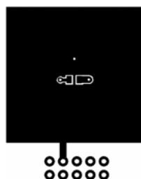
a) 80^\circ\text{C}/\text{W} when mounted on a 1\ \text{in}^2 pad of 2 oz copper
