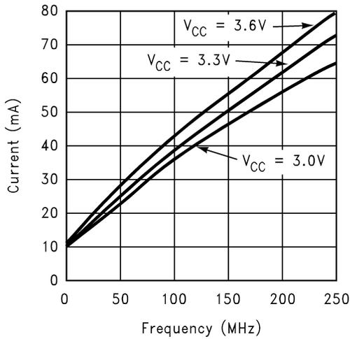
Figure 6. ICC vs Frequency, four channels switching
