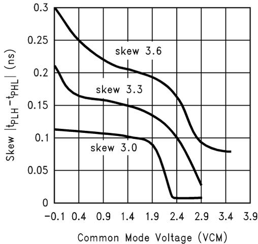
Figure 8. Typical Pulse Skew variation versus common-mode voltage
