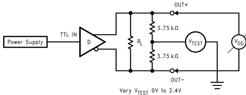
Figure 3. Differential Driver Full Load DC Test Circuit
