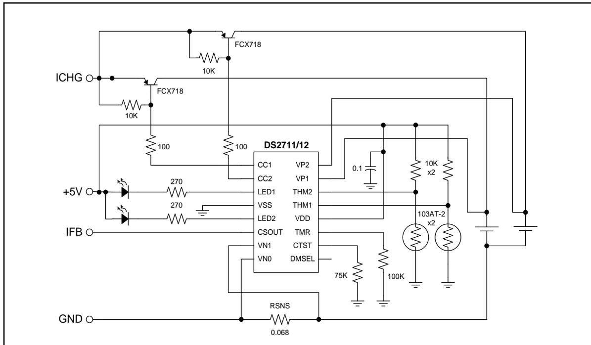
The series or parallel charge configuration is programmed by strapping LED2 in the low, high, or high-Z state during power-up. In this example and the following one, the parallel charge mode is selected by pulling LED2 pin high during power-up. This is accomplished in this example by the LED and 270Ω resistor. In applications where only one LED is used, a 100kΩ pullup resistor is recommended. See Table 2 for additional configuration programming information.
