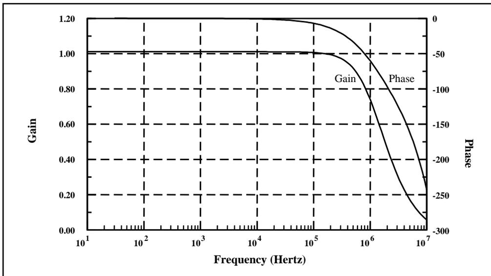
The open-loop amplifier response shown in Figure 6 was measured with  $I_{CSOUT} = -1\text{mA}$ . An error signal between the current-sense signal (across a sense resistor) and the 0.125V internal reference is produced so the voltage across the sense resistor is maintained at  $V_{IREF}$  in a closed-loop circuit.
