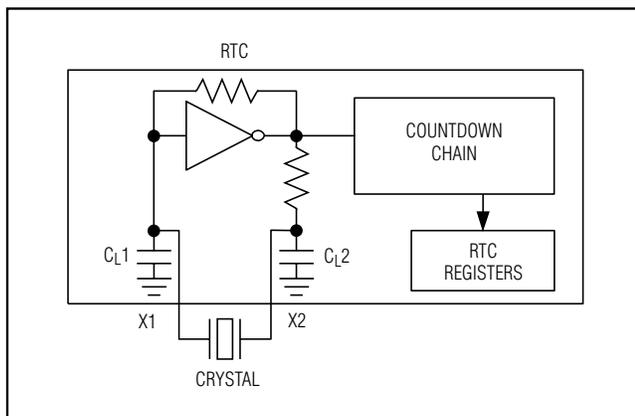
Figure 3. Oscillator Circuit Showing Internal Bias Network
