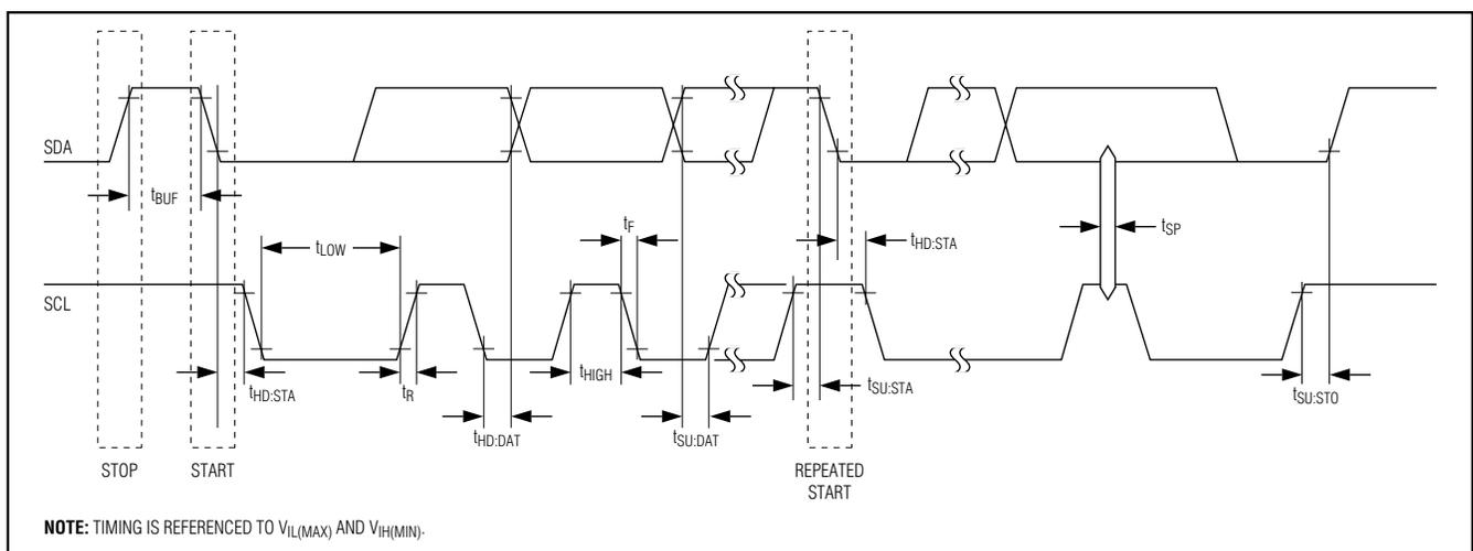
Figure 1. Data Transfer on I<sup>2</sup>C Serial Bus
