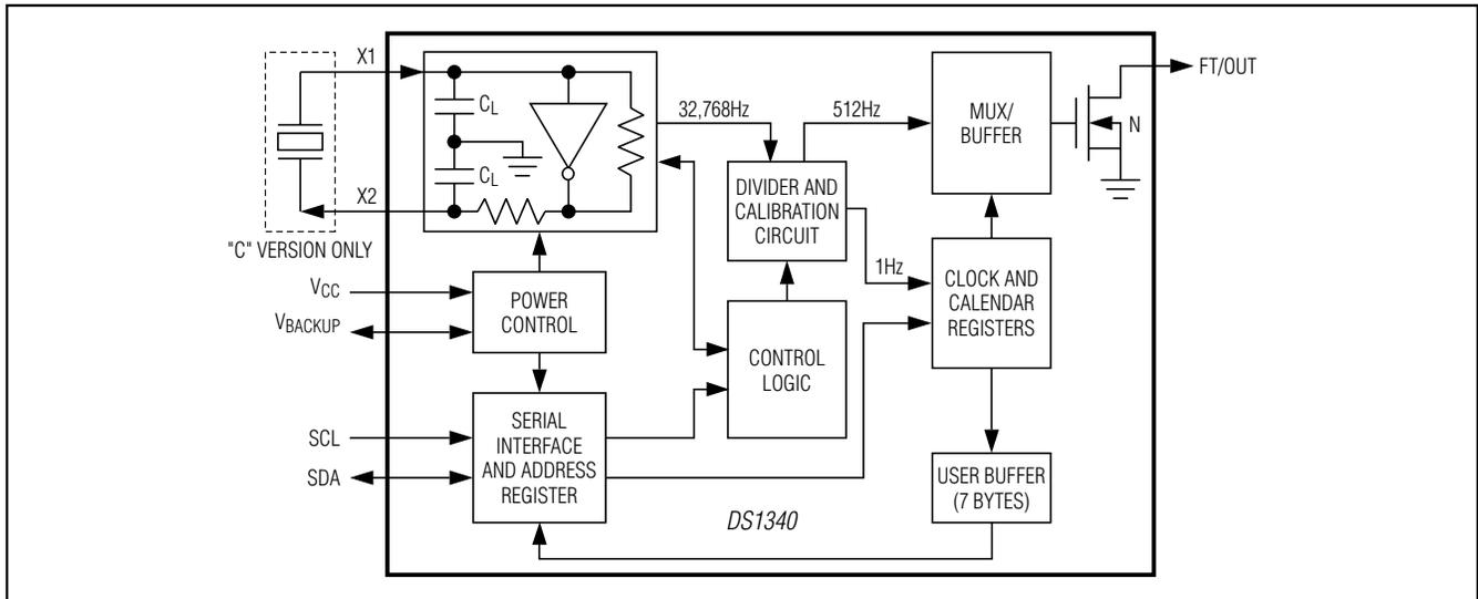
Figure 5. Functional Diagram
