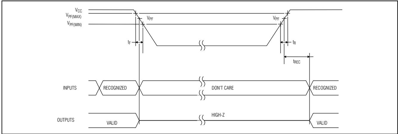
Figure 2. Power-Up/Power-Down Timing
