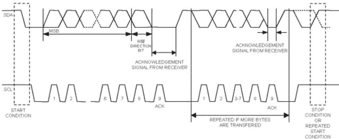
Depending upon the state of the  $\overline{R/W}$  bit, two types of data transfer are possible:
