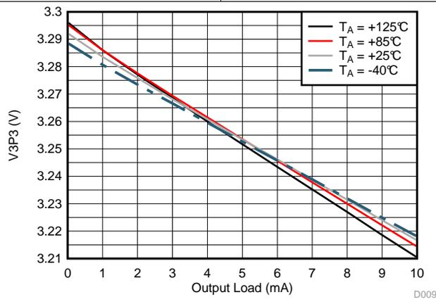
Figure 10. V3P3 Regulator vs Load at  $V_M = 24$  V
