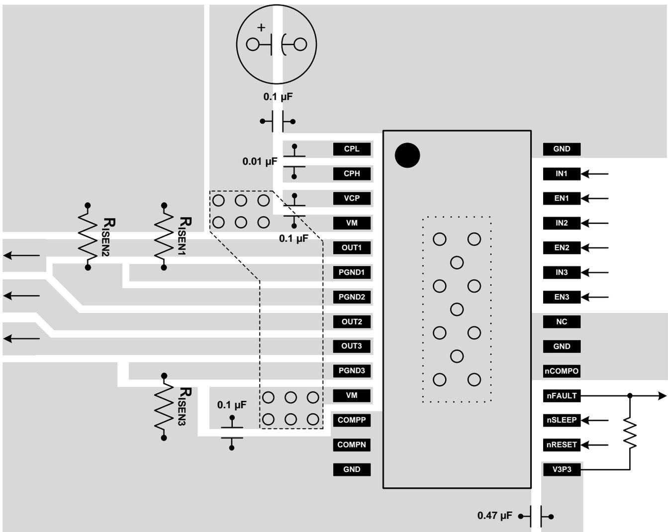
Figure 19. Recommended Layout Example For HTSSOP PWP Package
