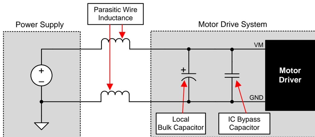
**Figure 18. Example Setup of Motor Drive System With External Power Supply**
