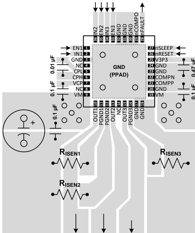
Figure 20. Recommended Layout Example For QFN RHH Package
