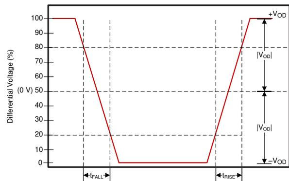
$V_{CM}$  is removed when the signals are viewed differentially.
