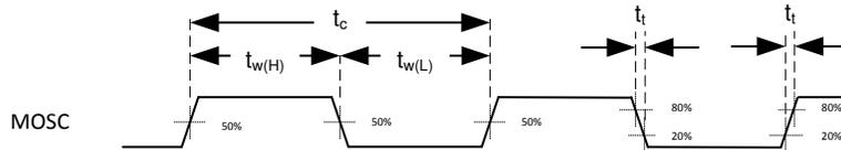
Figure 6-5. System Oscillators
