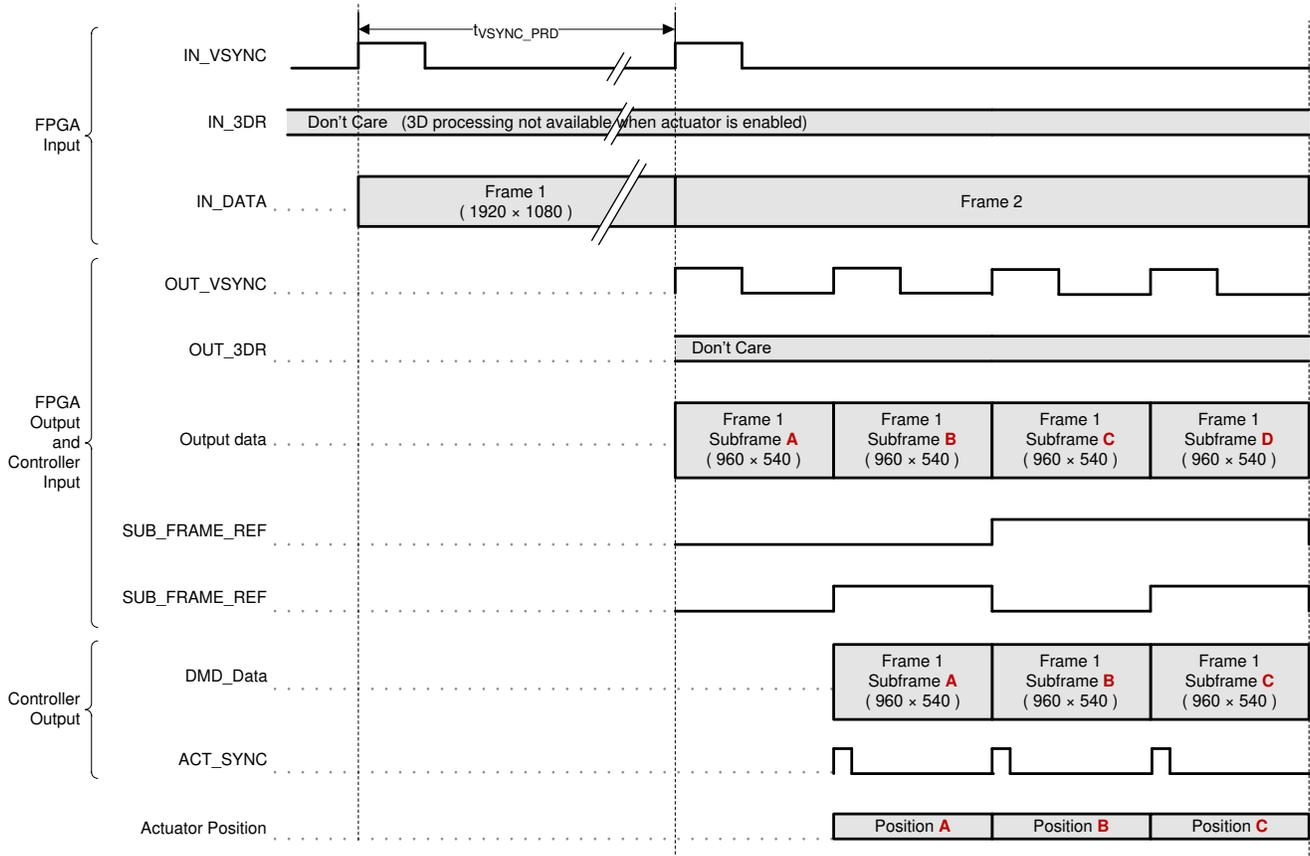
Figure 7-1. 2D Actuator Frame and Signal Timing
