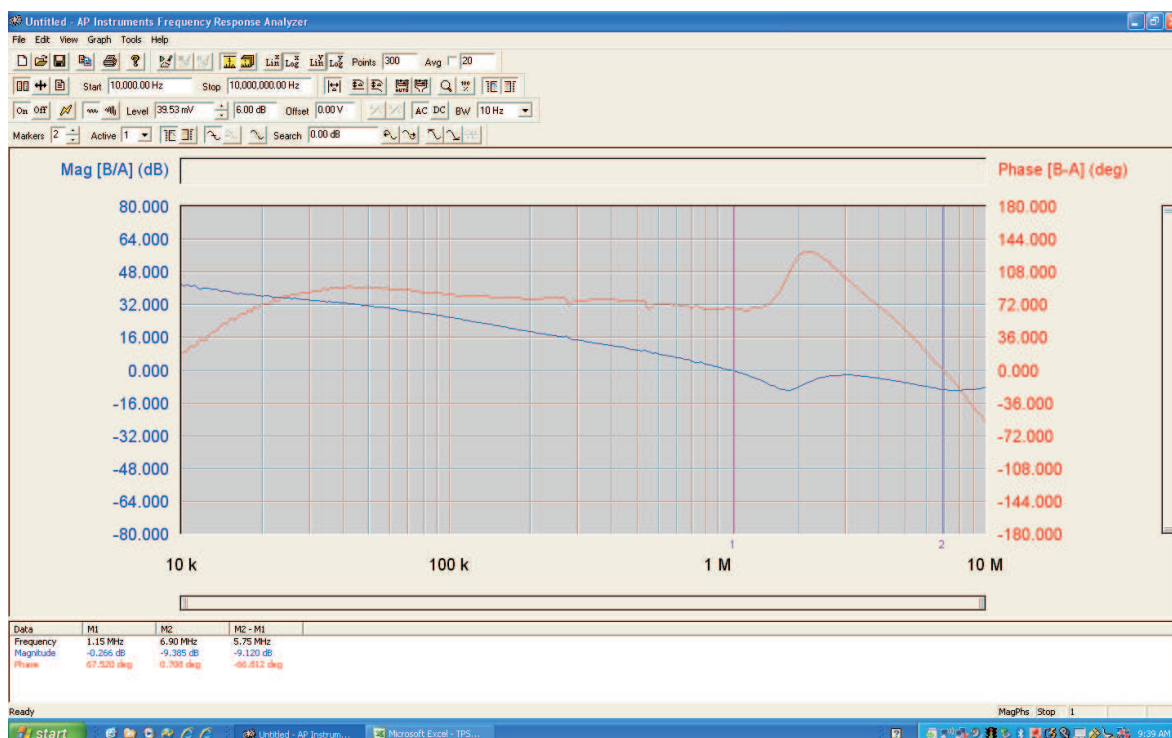
Figure 22. DDR3 VTT Bode Plot at 12 Vin, 1.5 VDDQ/0 A and VTT 1-A Sourcing
