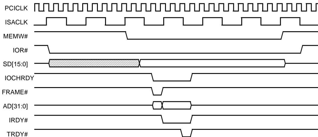
**Figure 3-13. ISA DMA Write To PCI Memory**
