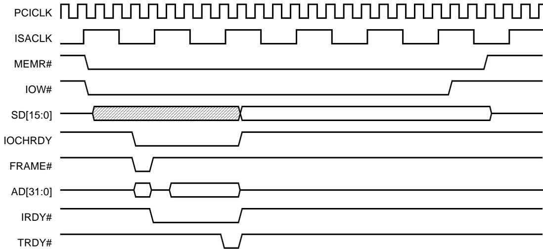
**Figure 3-12. ISA DMA Read from PCI Memory**
