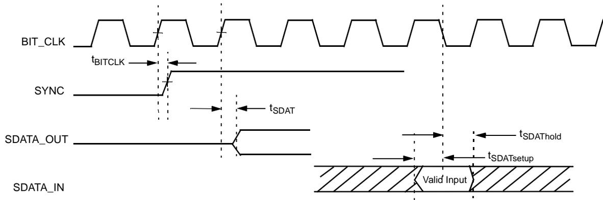
**Figure 5-5. Audio Interface Timing**
