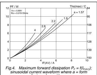
Fig.4. Maximum forward dissipation  $P_F = f(I_{F(AV)})$ ; sinusoidal current waveform where a = form factor =  $I_{F(RMS)} / I_{F(AV)}$ .
