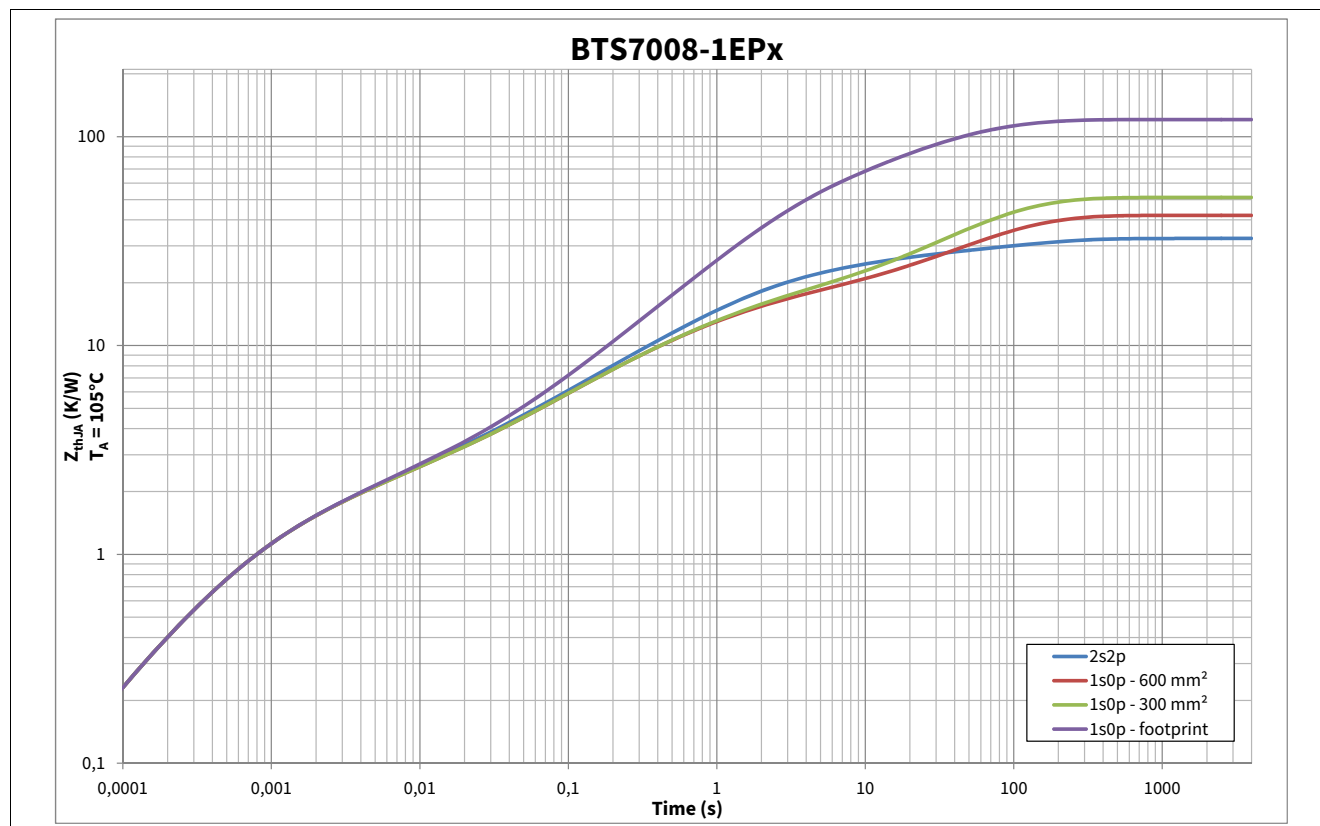
Figure 9 Typical Thermal Impedance. PCB setup according Chapter 4.4.1
