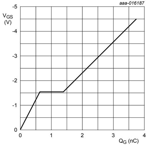
$I_D = -2 \text{ A}; V_{DS} = -10 \text{ V}; T_{amb} = 25 \text{ }^\circ\text{C}$
