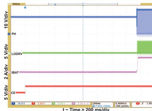
Figure 3. Charge Enable
