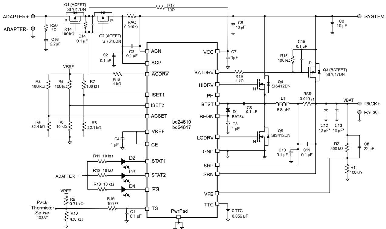
VIN=19V, 3-cell, I<sub>adapter\_limit</sub>=4A, I<sub>charge</sub>=3A, I<sub>pre-charge</sub>= I<sub>term</sub>=0.3A, 5 hour safety timer
