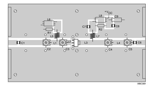
The circuit and components are situated on one side of a copper-clad PTFE fibre-glass board; the other side is unetched and serves as a ground plane. Earth connections from the component side to the ground plane are made by means of fixing screws, hollow rivets and copper foil straps, as shown.
