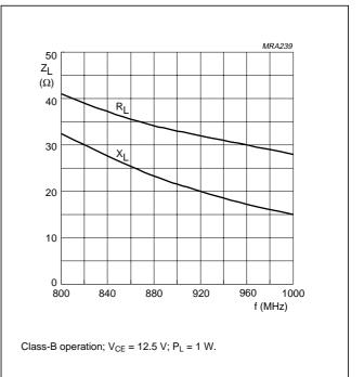
Fig.10 Load impedance (series components) as a function of frequency, typical values.
