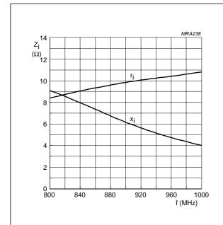
Class-B operation;  $V_{CE}$  = 12.5 V;  $P_L$  = 1 W.
