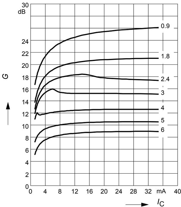
Power gain  $G_{ma}, G_{ms} = f(V_{CE})$
