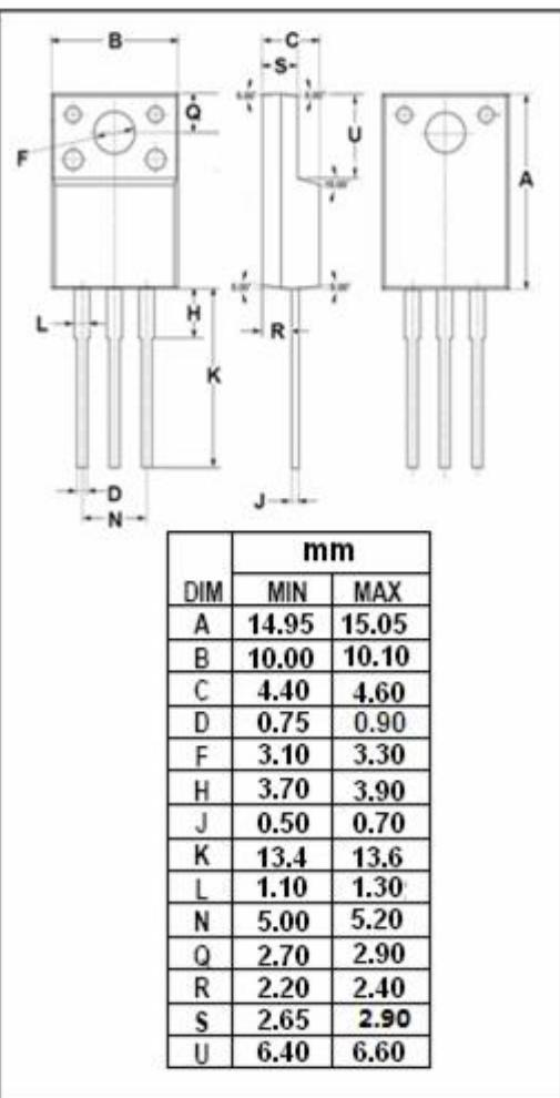
**isc Silicon NPN Darlington Power Transistor****BDW93CFP****ELECTRICAL CHARACTERISTICS****T<sub>c</sub>=25°C unless otherwise specified**
