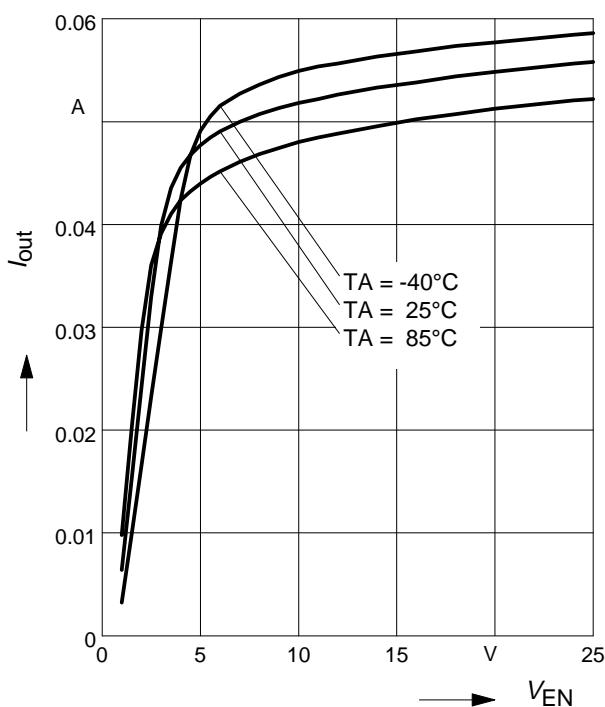
**BCR320U: Output current versus  $V_{\text{EN}}$**
