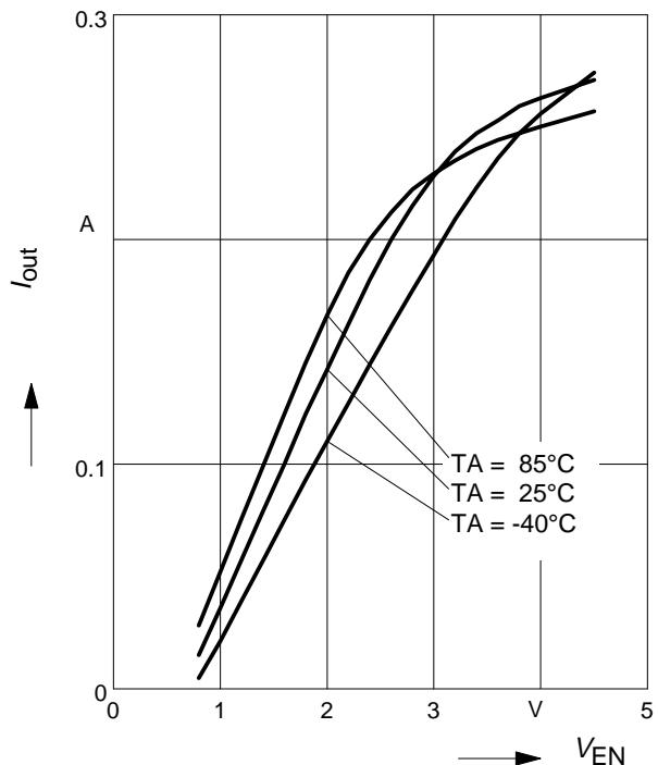
**BCR321U: Output current versus  $V_{EN}$**
