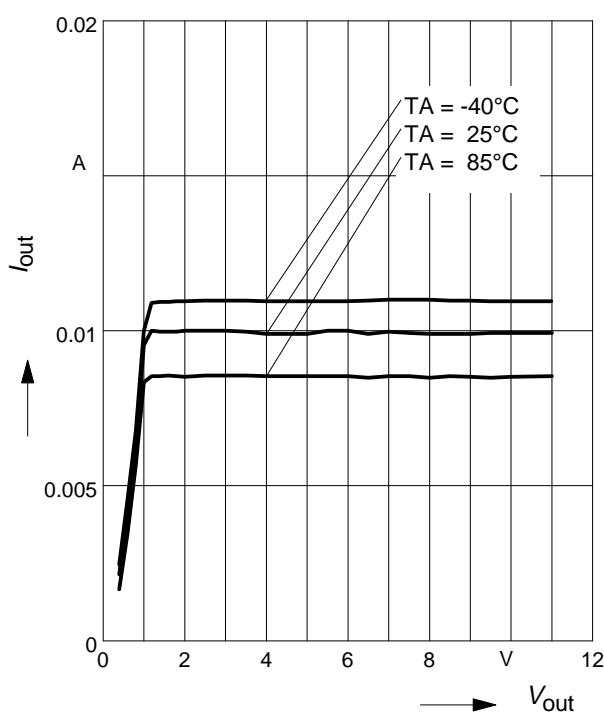
**BCR320U: Output current versus  $V_{out}$**
