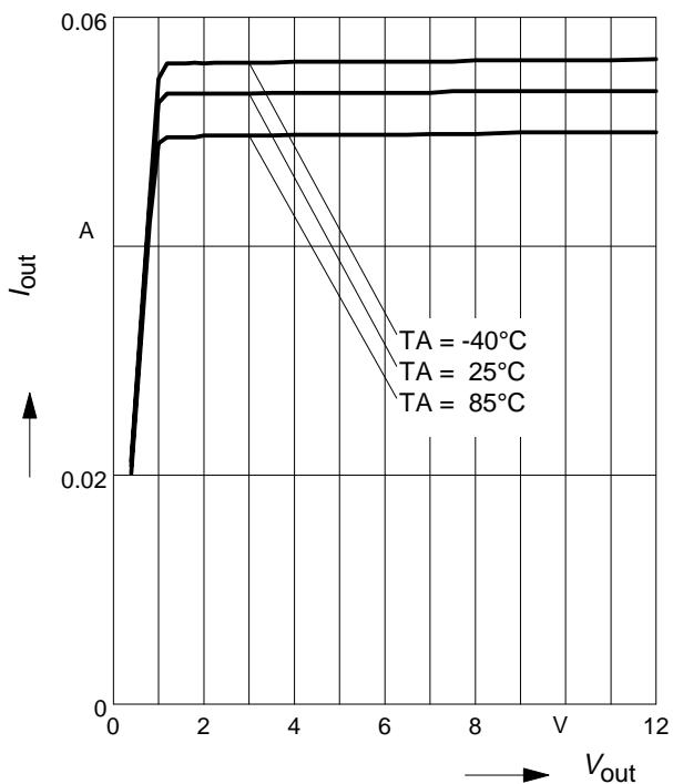
**BCR321U: Output current versus  $V_{out}$**
