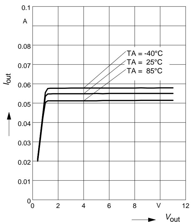
**BCR320U: Output current versus  $V_{\text{out}}$**
