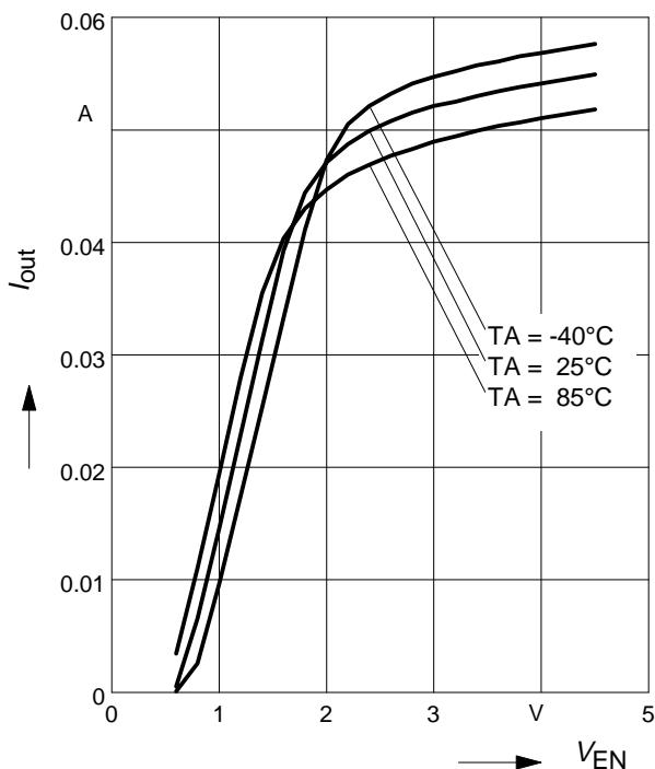
**BCR321U: Output current versus  $V_{EN}$**
