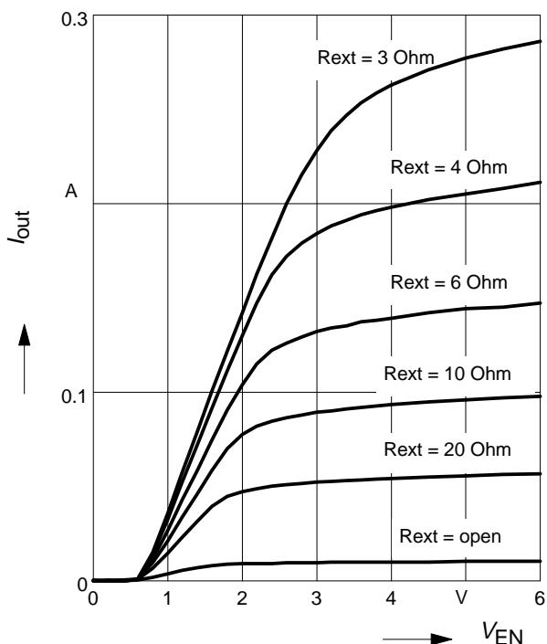
**BCR321U: Enable current versus  $V_{EN}$**
