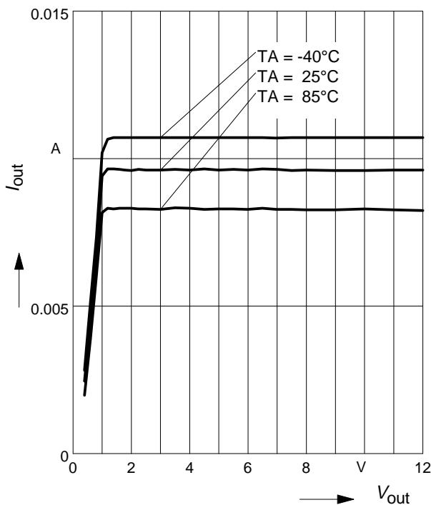
**BCR321U: Output current versus  $V_{out}$**
