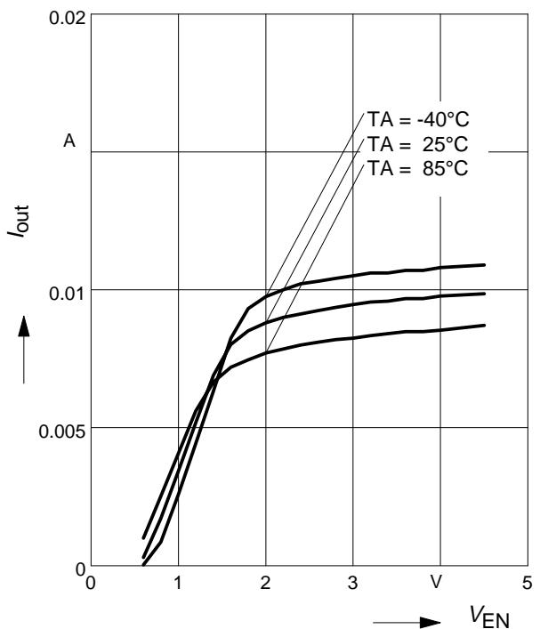
**BCR321U: Output current versus  $V_{EN}$**
