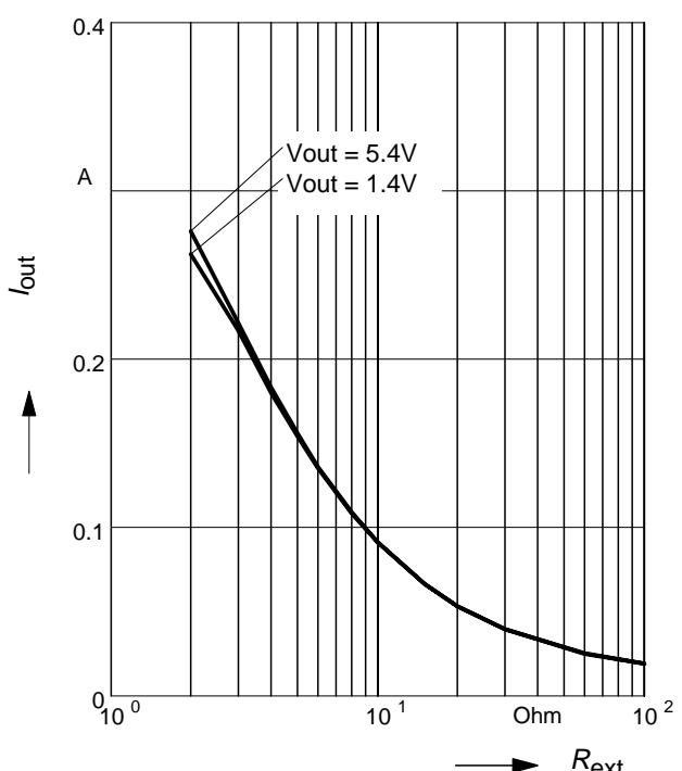
**BCR321U: Output current versus  $V_{out}$**
