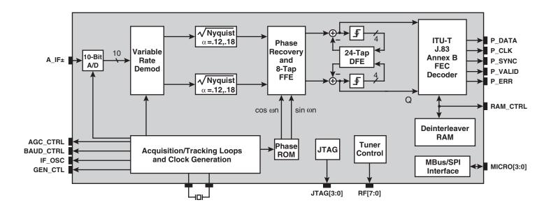
The **BCM3116** QAMLink Receiver is a fully asynchronous design with an integrated FEC and 10-bit analog-to-digital converter. It provides a complete digital transmission solution for cable modems, cable-TV set-top boxes and digital microwave radios. Its bandwidth-efficient feature set expands the existing potential bandwidth of a standard analog network and provides operators with reliable, error-free transmission.
