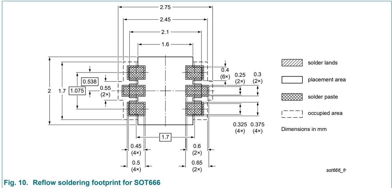
Fig. 10. Reflow soldering footprint for SOT666
