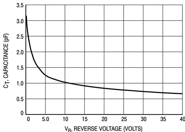
Figure 3. Typical Capacitance
