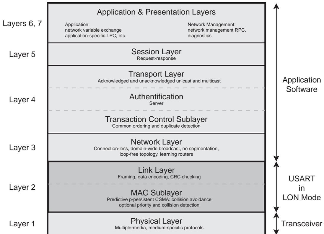
The USART configured in LON mode is a full-layer 2 implementation including standard timings handling, framing (transmit and receive PPDU frames), backlog estimation and other features. At the frame encoding/decoding level, differential Manchester encoding is used (also known as CDP).
