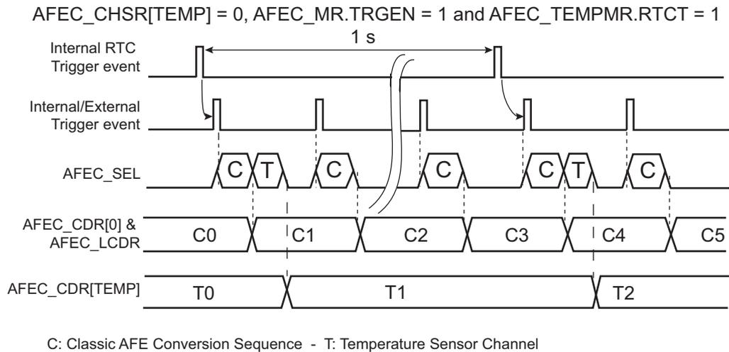
Assuming AFEC\_CHSR[0] = 1 and AFEC\_CHSR[TEMP] = 1 where TEMP is the index of the temperature sensor channel
