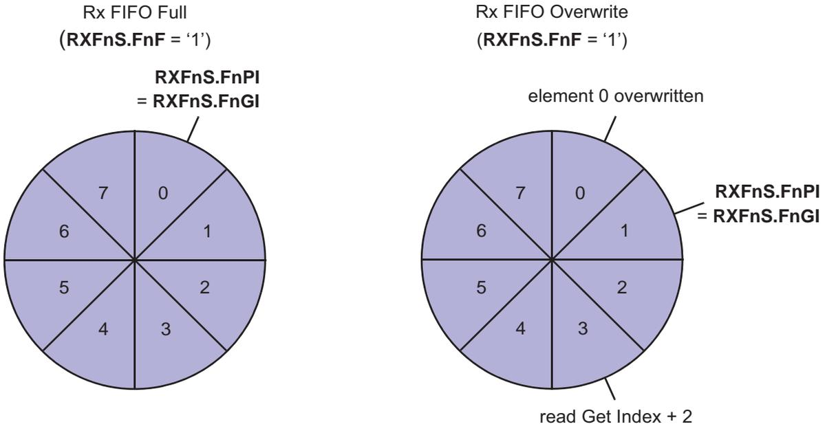
After reading from the Rx FIFO, the number of the last element read has to be written to the Rx FIFO Acknowledge Index  $\text{RXFnA.FnA}$ . This increments the get index to that element number. In case the put index has not been incremented to this Rx FIFO element, the Rx FIFO full condition is reset ( $\text{MCAN\_RXFnS.FnF} = '0'$ ).
