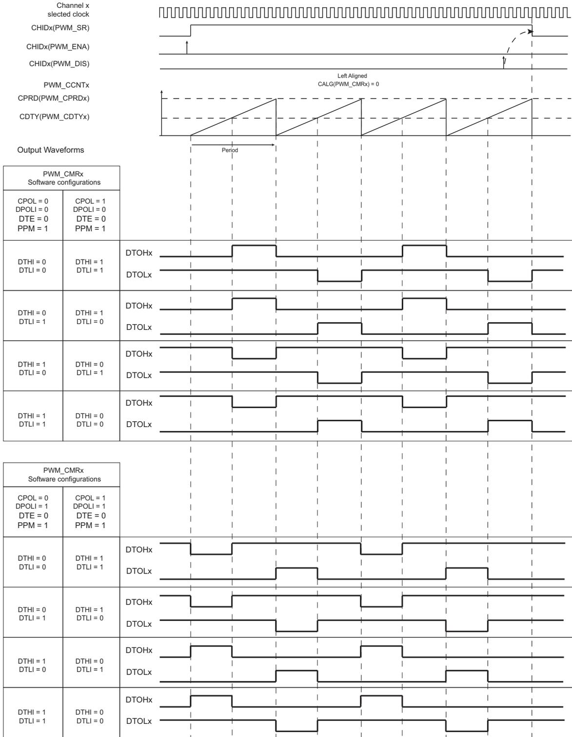
**Figure 49-12. PWM Push-Pull Waveforms: Center-Aligned Mode**
