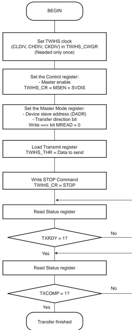
**Figure 42-15. TWIHS Write Operation with Single Data Byte and Internal Address**
