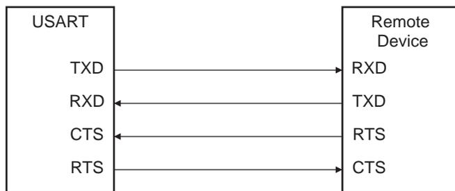
Setting the USART to operate with hardware handshaking is performed by writing the USART\_MODE field in US\_MR to the value 0x2.
