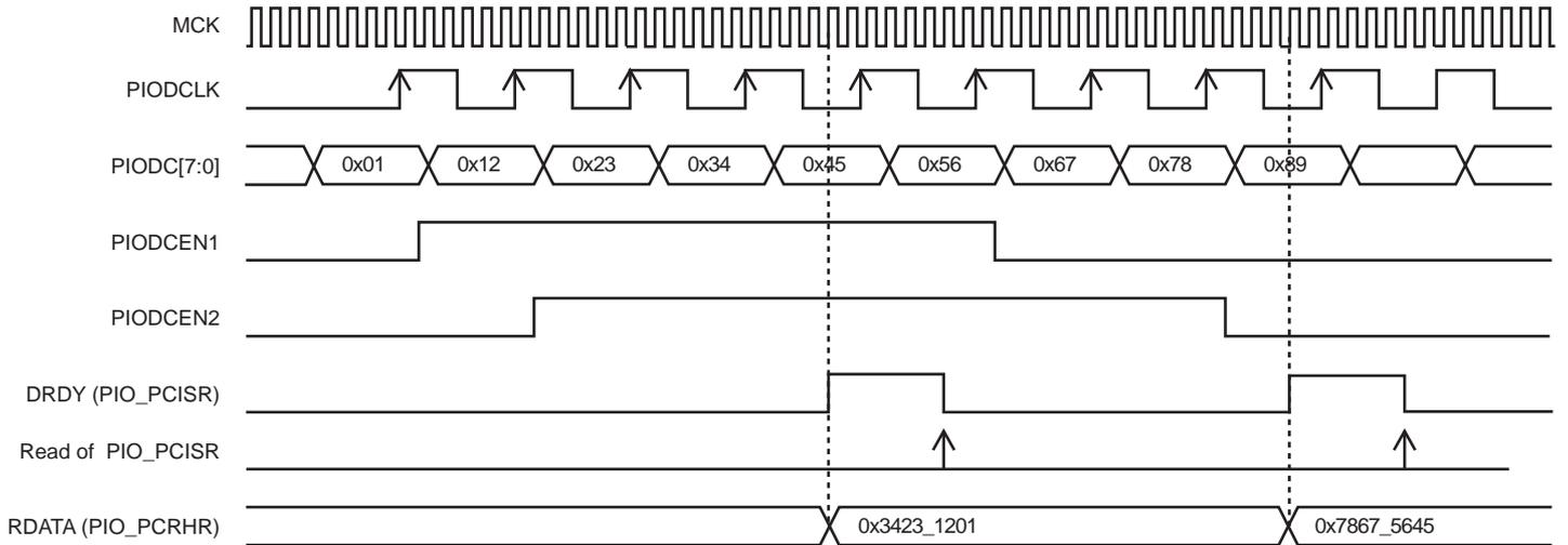
**Figure 32-11. Parallel Capture Mode Waveforms (DSIZE = 2, ALWAYS = 0, HALFS = 1, FRSTS = 0)**
