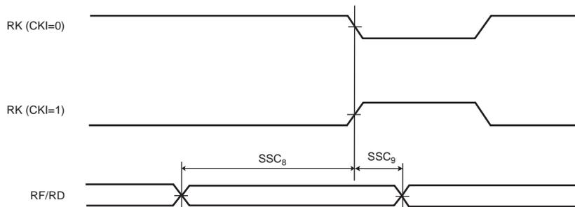
**Figure 56-64. SSC Receiver, RK in Input and RF in Output**
