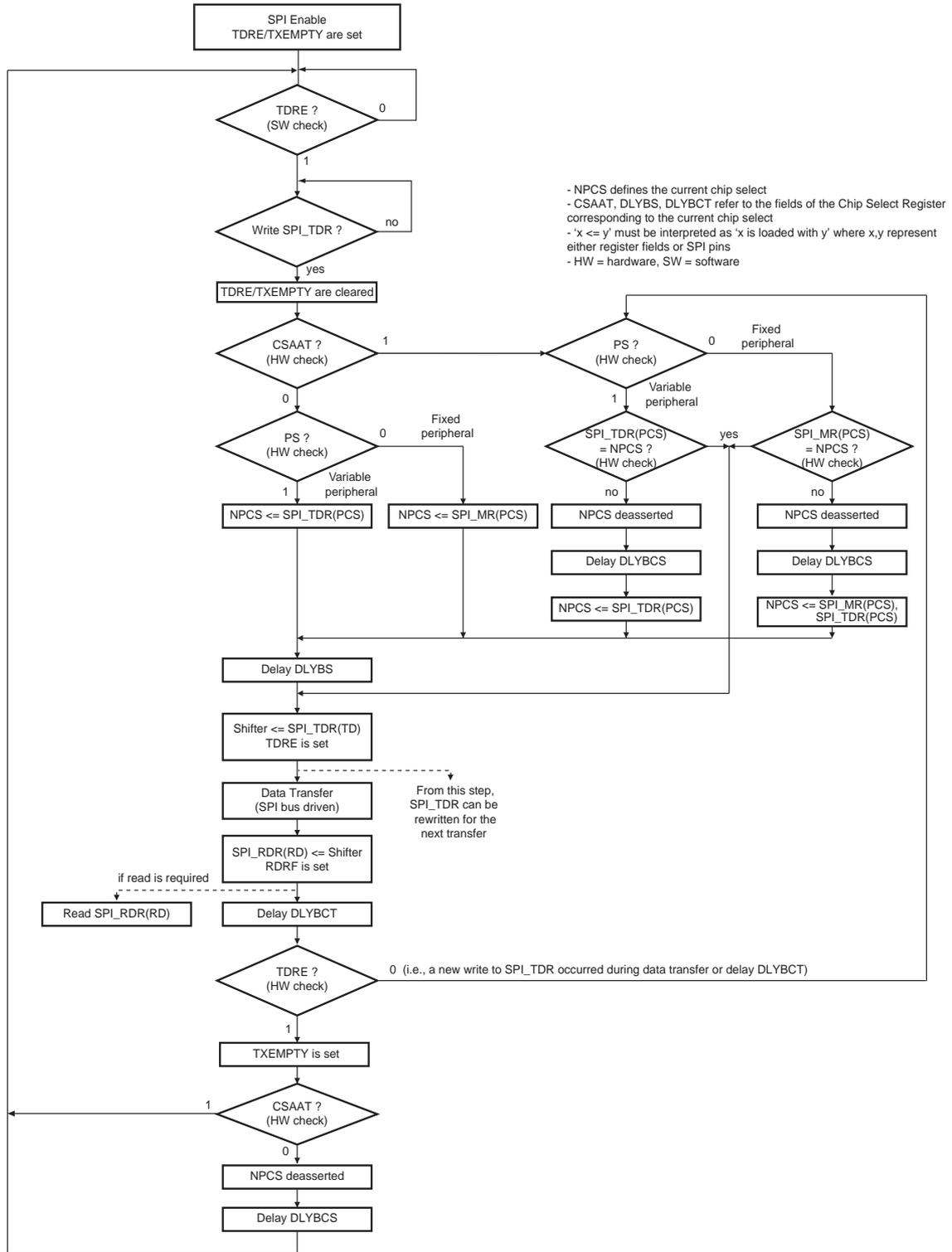
Figure 40-8 shows the behavior of Transmit Data Register Empty (TDRE), Receive Data Register (RDRF) and Transmission Register Empty (TXEMPTY) status flags within the SPI\_SR during an 8-bit data transfer in Fixed mode without the DMA involved.
