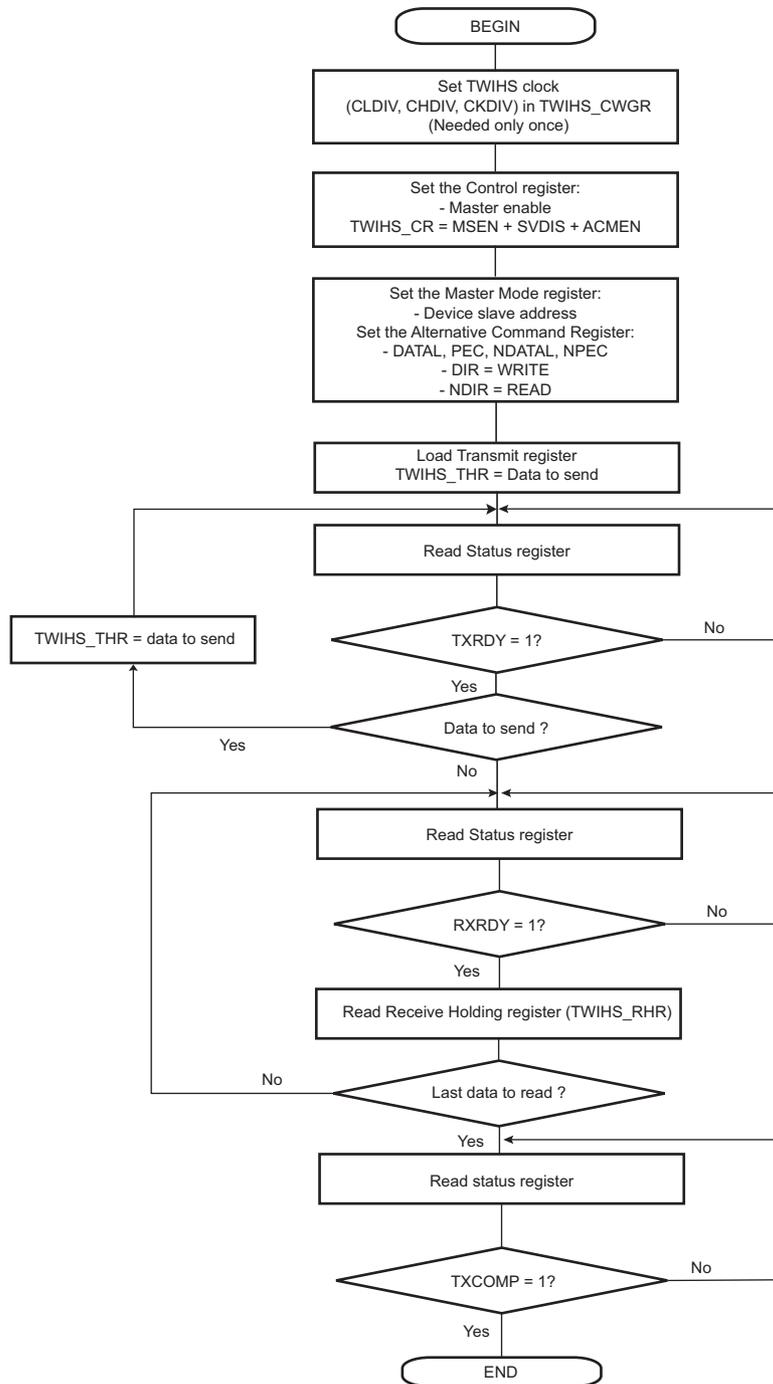
Figure 42-21. TWIHS Read Operation with Single Data Byte without Internal Address
