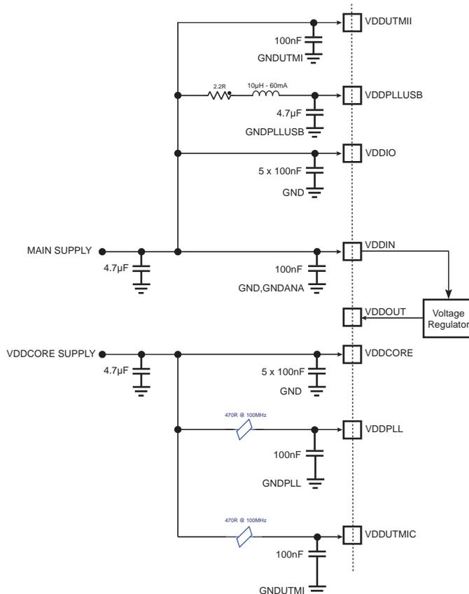
Note: Component values are given only as a typical example
