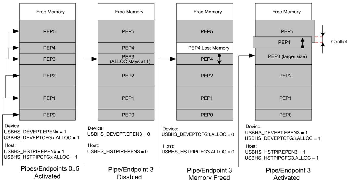
1. Pipes/endpoints 0 to 5 are enabled, configured and allocated in ascending order. Each pipe/endpoint then owns a memory area in the DPRAM.
