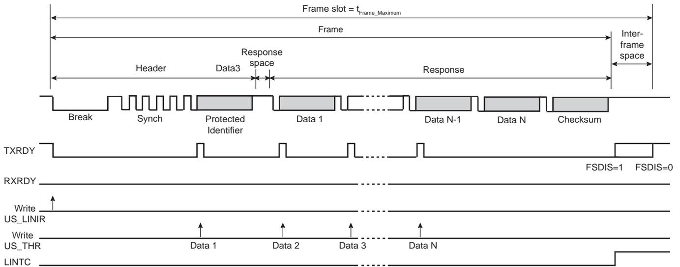
**Figure 45-46. Master Node Configuration, NACT = SUBSCRIBE**
