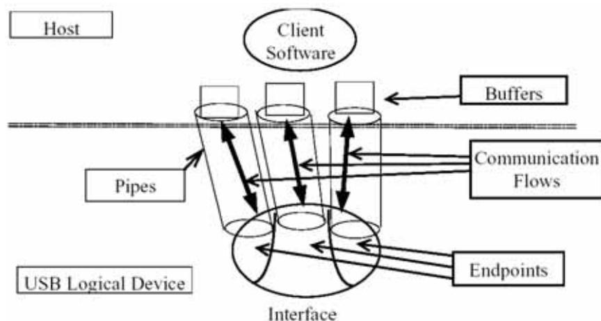
In Host mode, the USBHS associates a pipe to a device endpoint, considering the device configuration descriptors.
