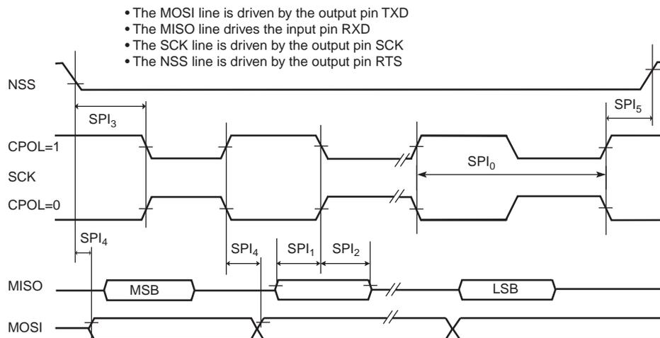
**Figure 56-53. USART SPI Slave Mode (Mode 1 or 2)**
