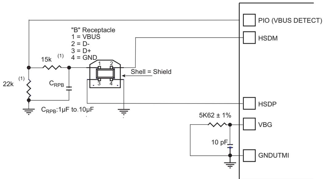
Note: The values shown on the 22 k $\Omega$  and 15 k $\Omega$  resistors are only valid with 3.3V supplied PIOs.
