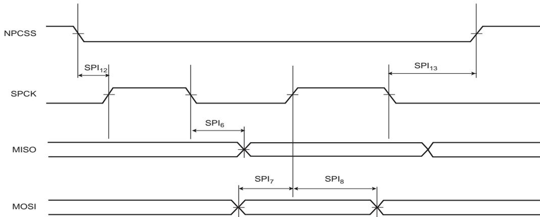
**Figure 56-49. SPI Slave Mode with (CPOL = NCPHA = 0) or (CPOL= NCPHA= 1)**
