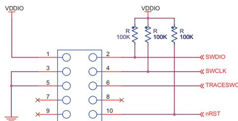
Figure 58-2. SWD Schematic Example with a 20-pin Connector
