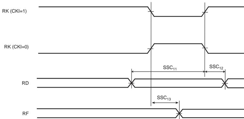
**Figure 56-40. SSC Receiver, RK in Output and RF in Input**
