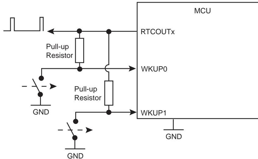
**Figure 22-10. Low-power Debouncer (Push-to-Break Switch, Pull-down Resistors)**
