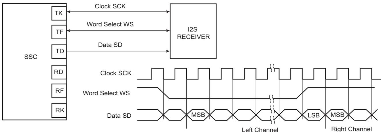
**Figure 43-4. Codec Application Block Diagram**
