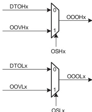
The fields OSHx and OSLx in the [PWM Output Selection Register](#) (PWM\_OS) allow the outputs of the dead-time generator DTOHx and DTOLx to be overridden by the value defined in the fields OOVHx and OOVLx in the [PWM Output Override Value Register](#) (PWM\_OOV).
