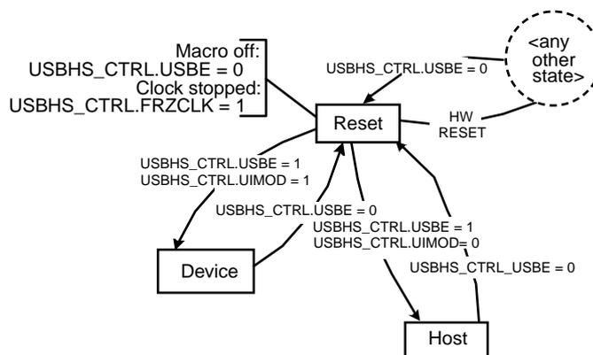
After a hardware reset, the USBHS is in Reset state. In this state:
