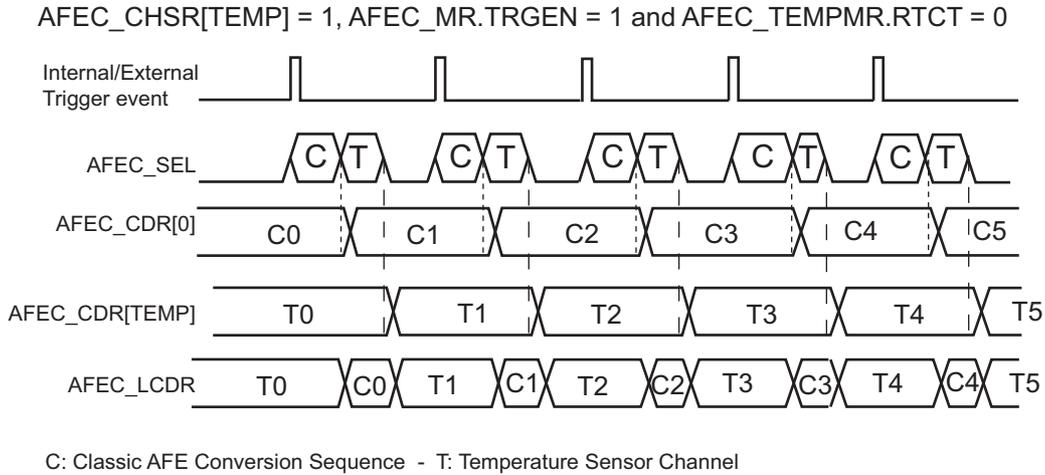
Assuming AFEC\_CHSR[0] = 1 and AFEC\_CHSR[TEMP] = 1 where TEMP is the index of the temperature sensor channel
