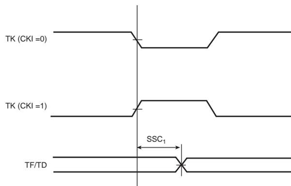
**Figure 56-61. SSC Transmitter, TK in Output and TF in Input**
