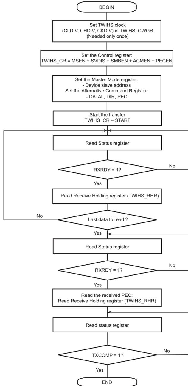
Figure 42-26. TWIHS Read Operation with Multiple Data Bytes + Write Operation with Multiple Data Bytes (Sr)
