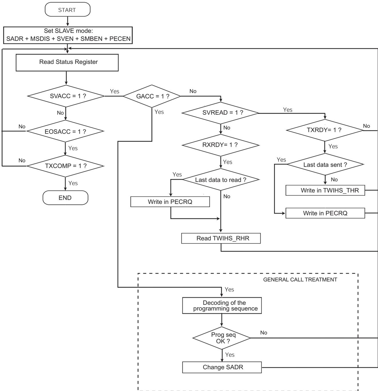
Figure 42-45. Read Write Flowchart in Slave Mode with SMBus PEC and Alternative Command Mode
