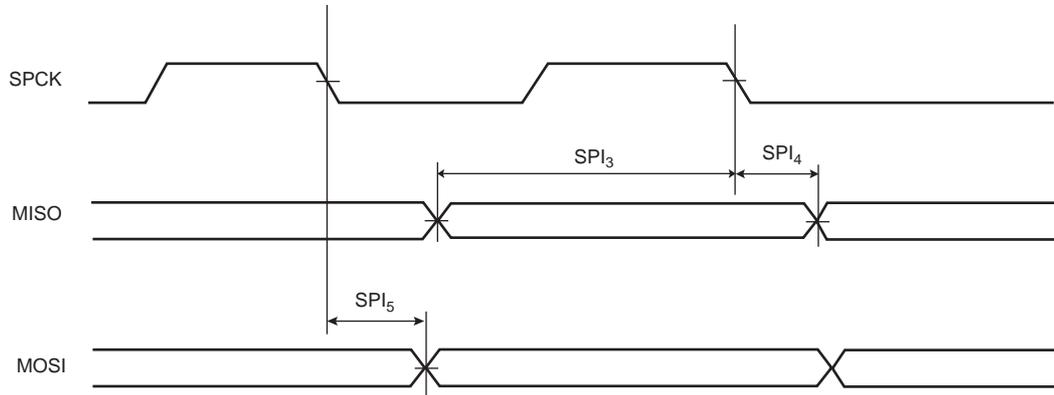
**Figure 56-48. SPI Slave Mode with (CPOL=0 and NCPHA=1) or (CPOL=1 and NCPHA=0)**
