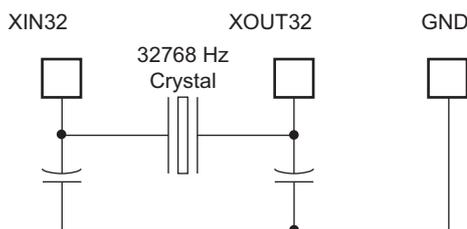
The 32.768 kHz crystal oscillator provides a more accurate frequency than the 32 kHz (typical) RC oscillator.
