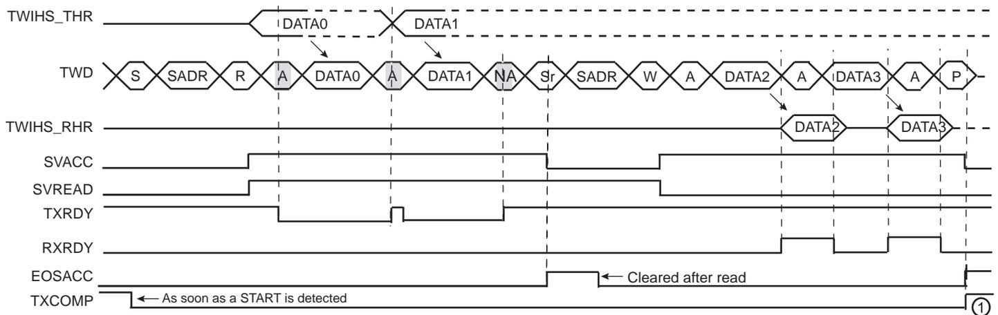
Note: TXCOMP is only set at the end of the transmission. This is because after the REPEATED START, SADR is detected again.
