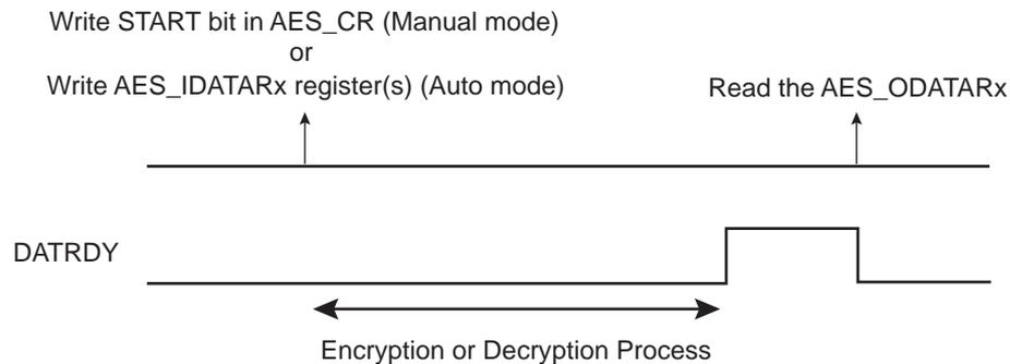
If the user does not want to read the AES\_ODATARx between each encryption/decryption, the DATRDY flag will not be cleared. If the DATRDY flag is not cleared, the user cannot know the end of the following encryptions/decryptions.
