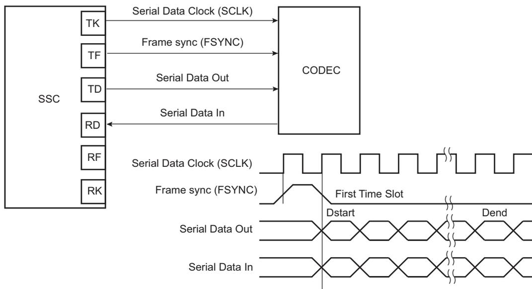
**Figure 43-5. Time Slot Application Block Diagram**
