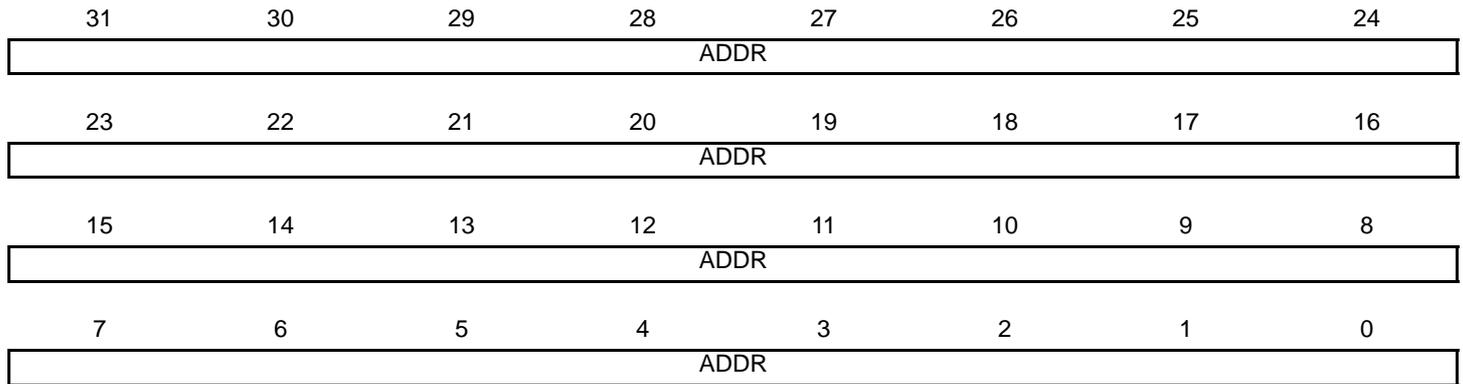
The unicast hash enable (UNIHEN) and the multicast hash enable (MITIHEN) bits in the [GMAC Network Configuration Register](#) enable the reception of hash matched frames. See [Section 38.6.9 "Hash Addressing"](#).
