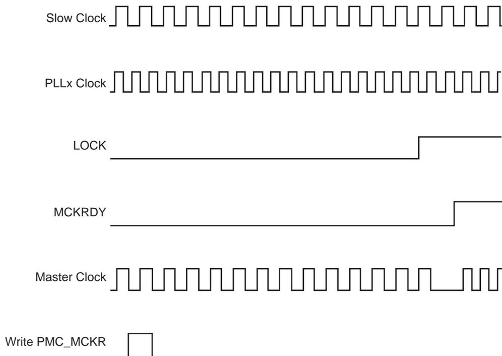
**Figure 31-7. Switch Master Clock from Main Clock to Slow Clock**
