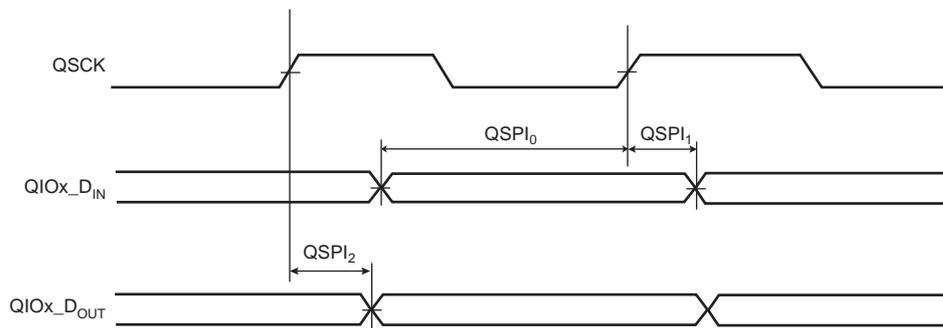
**Figure 56-18. QSPI Master Mode with (CPOL = 0 and NCPHA=1) or (CPOL=1 and NCPHA= 0)**
