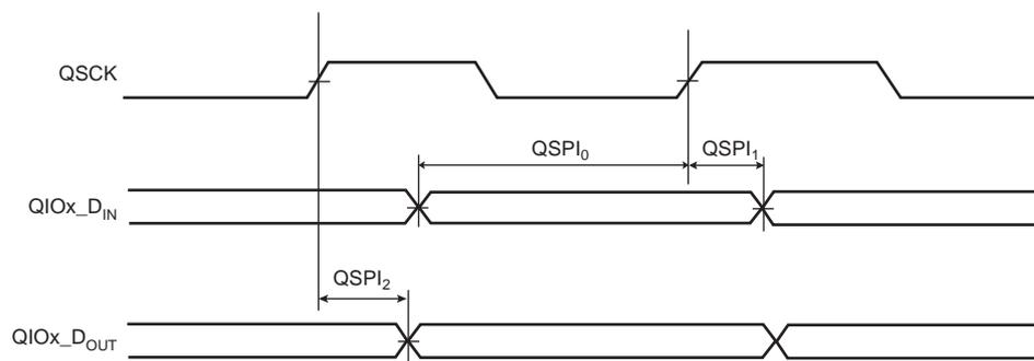
**Figure 56-44. QSPI Master Mode with (CPOL = 0 and NCPHA=1) or (CPOL=1 and NCPHA= 0)**
