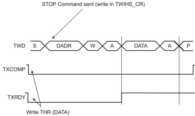
**Figure 42-5. Master Write with Multiple Data Bytes**
