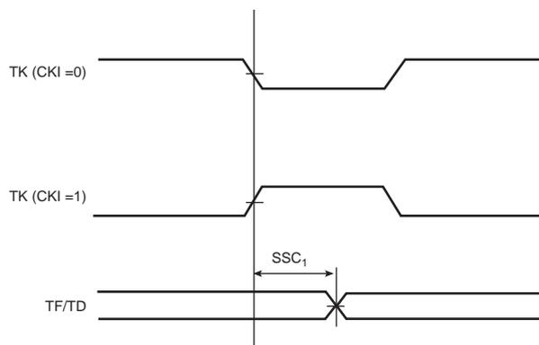
**Figure 56-35. SSC Transmitter, TK in Output and TF in Input**
