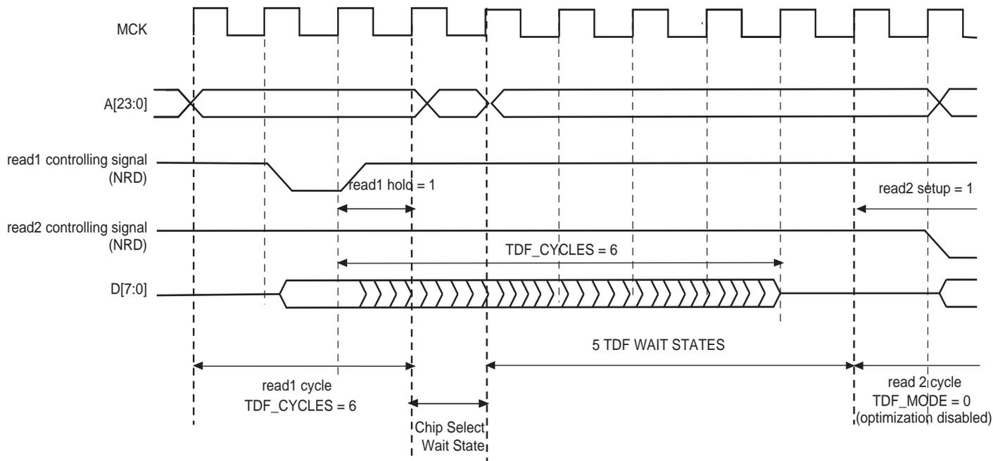
**Figure 34-23. TDF Mode = 0: TDF wait states between a read and a write access on different chip selects**
