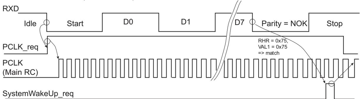
**Figure 46-14. Asynchronous Event Generating Only Partial Wake-up**
