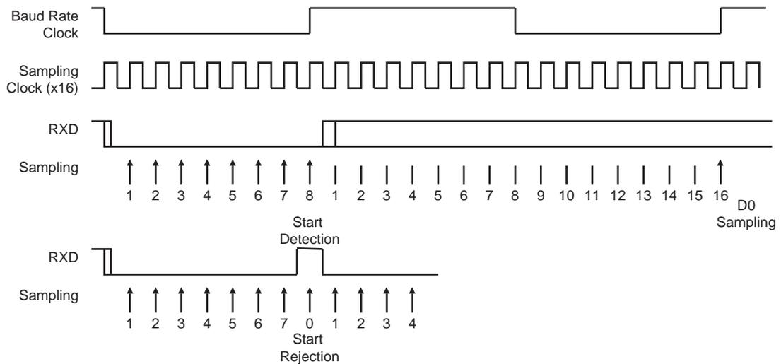
**Figure 45-12. Asynchronous Character Reception**
