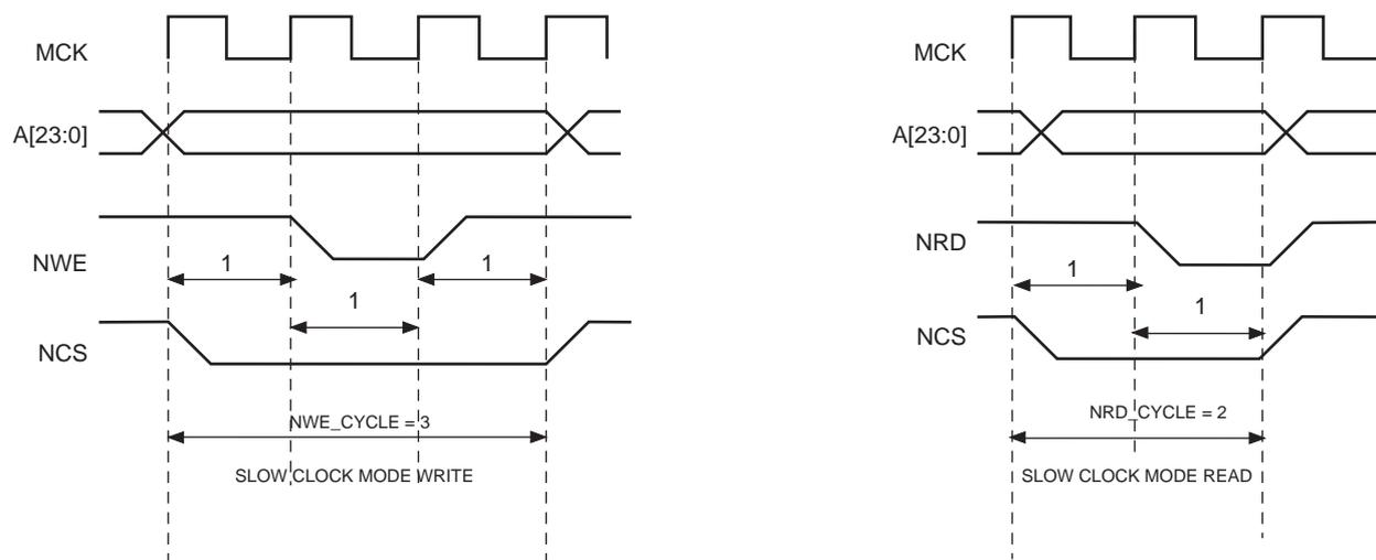
Table 34-7. Read and Write Timing Parameters in Slow Clock Mode
