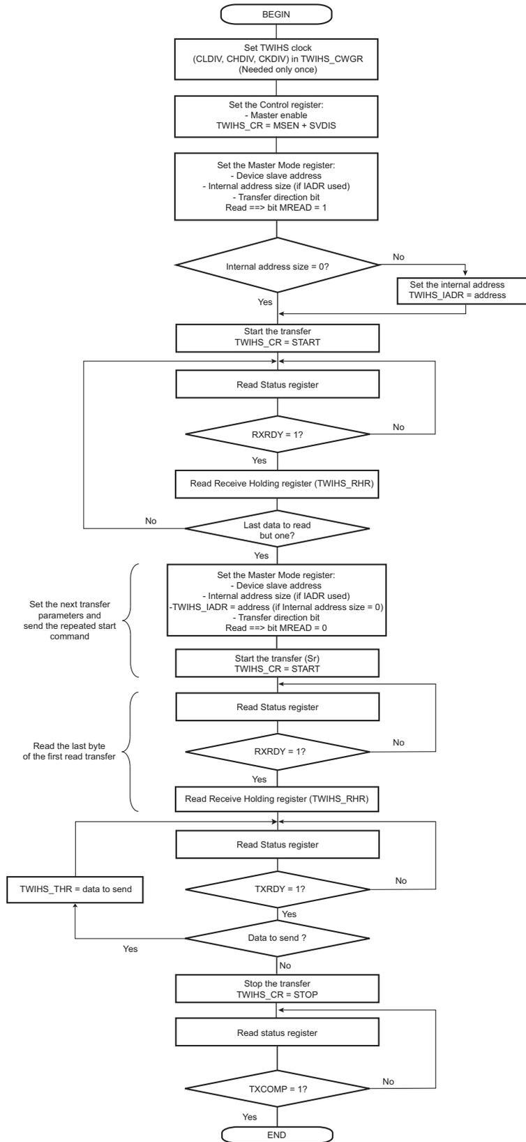
Figure 42-27. TWIHS Read Operation with Multiple Data Bytes + Write with Alternative Command Mode with PEC
