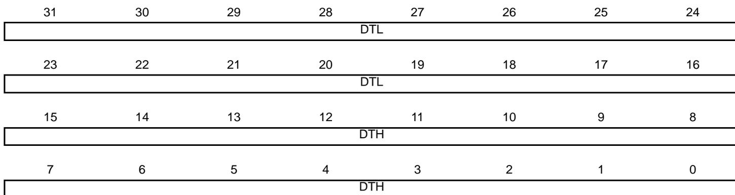
This register can only be written if bits WPSWS4 and WPHWS4 are cleared in the [PWM Write Protection Status Register](#). Only the first 12 bits (dead-time counter size) of fields DTH and DTL are significant.
