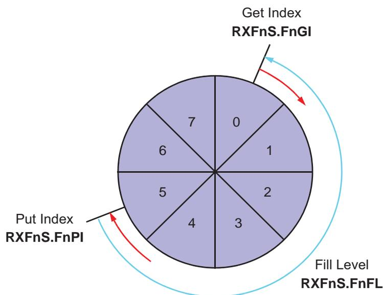
When reading from an Rx FIFO, Rx FIFO Get Index  $RXFnS.FnGI \times$  FIFO Element Size has to be added to the corresponding Rx FIFO start address  $RXFnC.FnSA$ .
