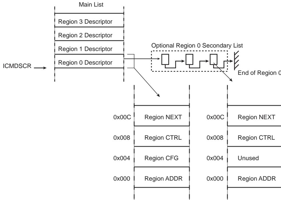
Figure 53-5 shows an example of the mandatory ICM settings to monitor three memory data blocks of the system memory (defined as two regions) with one region being not contiguous (two separate areas) and one contiguous memory area. For each said region, the SHA algorithm may be independently selected (different for each region). The wrap allows continuous monitoring.
