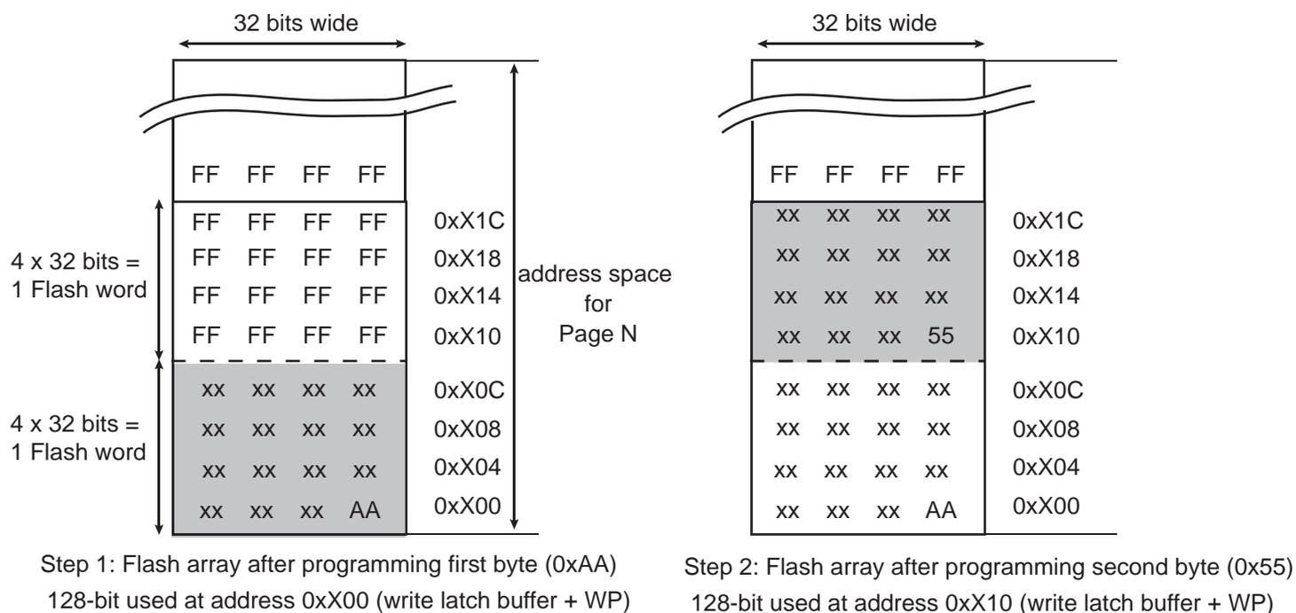
Note: The byte location shown here is for example only, it can be any byte location within a 64-bit word
