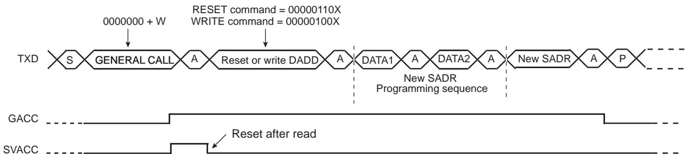
Note: This method enables the user to create a personal programming sequence by choosing the programming bytes and their number. The programming sequence has to be provided to the master.
