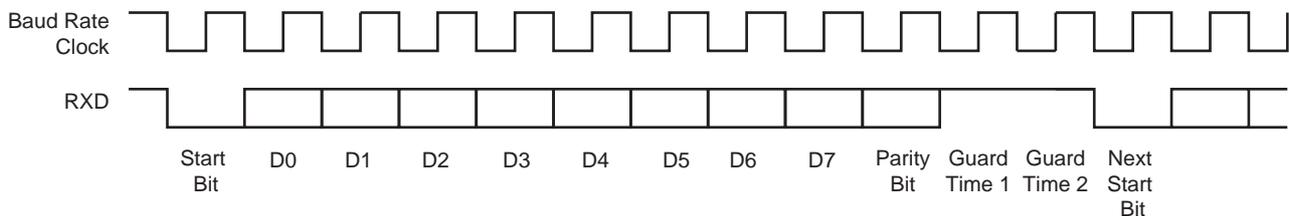
**Figure 45-31. T = 0 Protocol with Parity Error**
