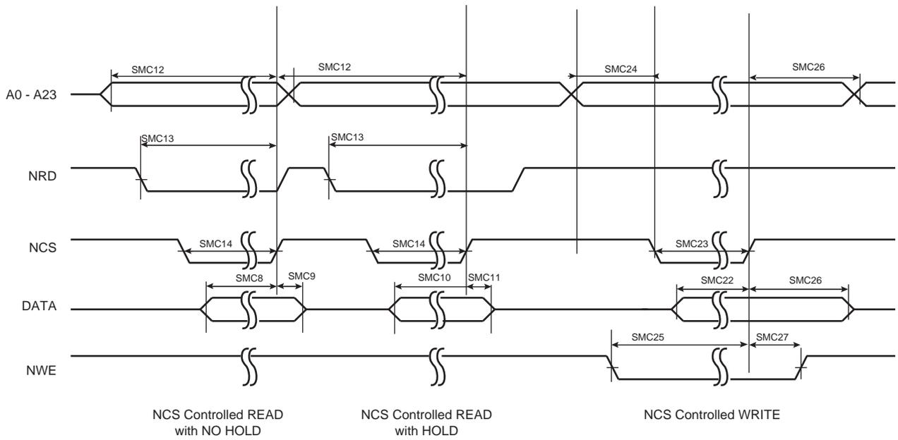
**Figure 56-51. SMC Timings - NRD Controlled Read and NWE Controlled Write**
