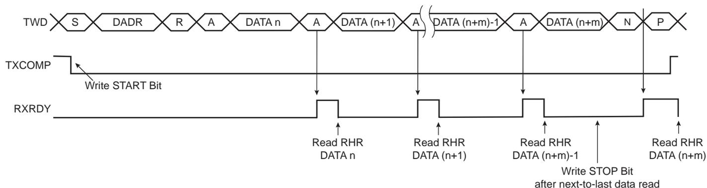
**Figure 42-9. Master Read Clock Stretching with Multiple Data Bytes**
