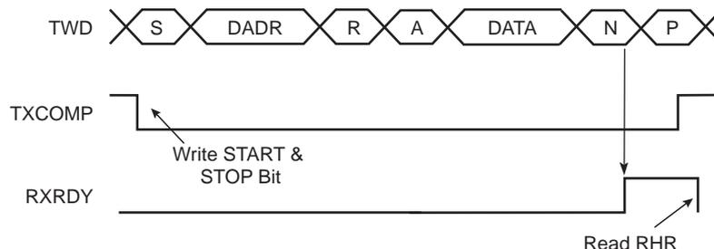
**Figure 42-8. Master Read with Multiple Data Bytes**
