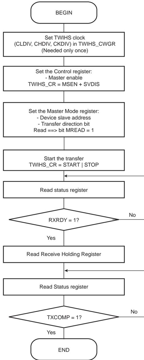
Figure 42-22. TWIHS Read Operation with Single Data Byte and Internal Address
