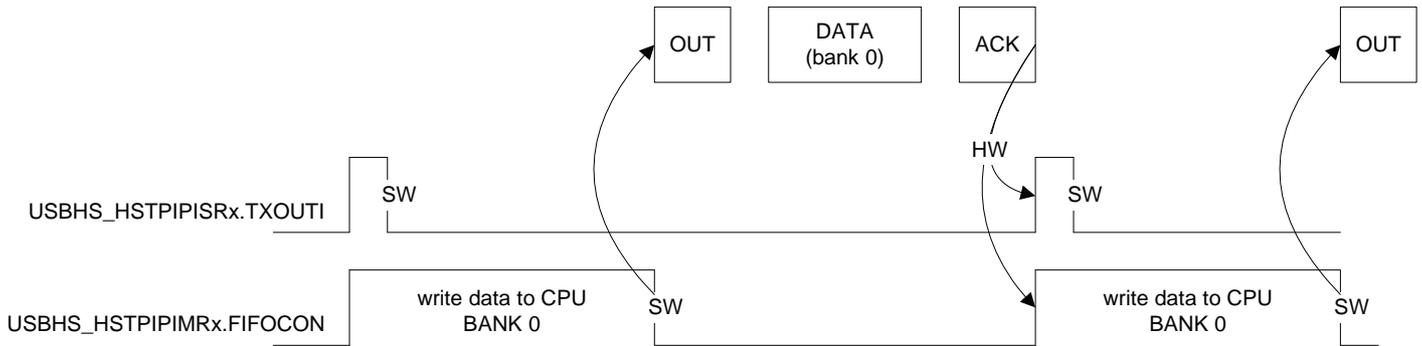
**Figure 37-22. Example of an OUT Pipe with two Data Banks and no Bank Switching Delay**
