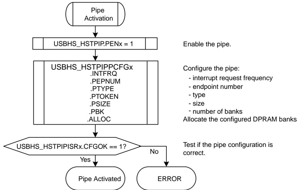
As long as the pipe is not correctly configured ( $USBHS\_HSTPIISRx.CFGOK = 0$ ), the controller cannot send packets to the device through this pipe.
