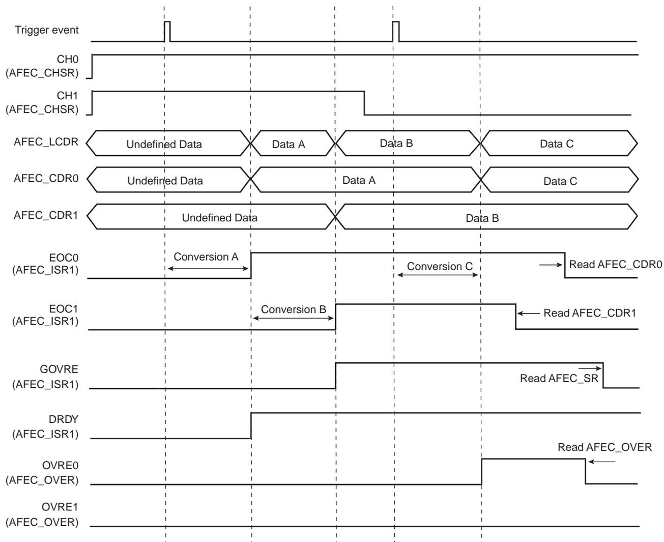
**Warning:** If the corresponding channel is disabled during a conversion, or if it is disabled and then reenabled during a conversion, its associated data and its corresponding EOCx and GOVRE flags in AFEC\_ISR and OVREx flags in AFEC\_OVER are unpredictable.
