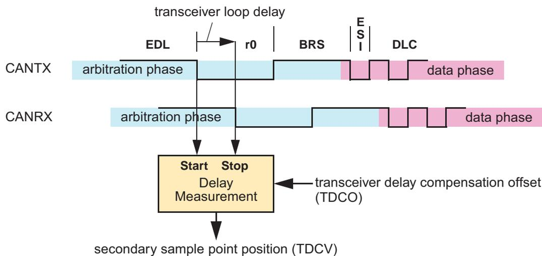
Within each CAN FD frame, the transmitter measures the delay between the data transmitted at pin CANTX and the data received at pin CANRX. The measurement is done once, at the falling edge of bit EDL to bit r0. The delay is measured in CAN core clock periods.
