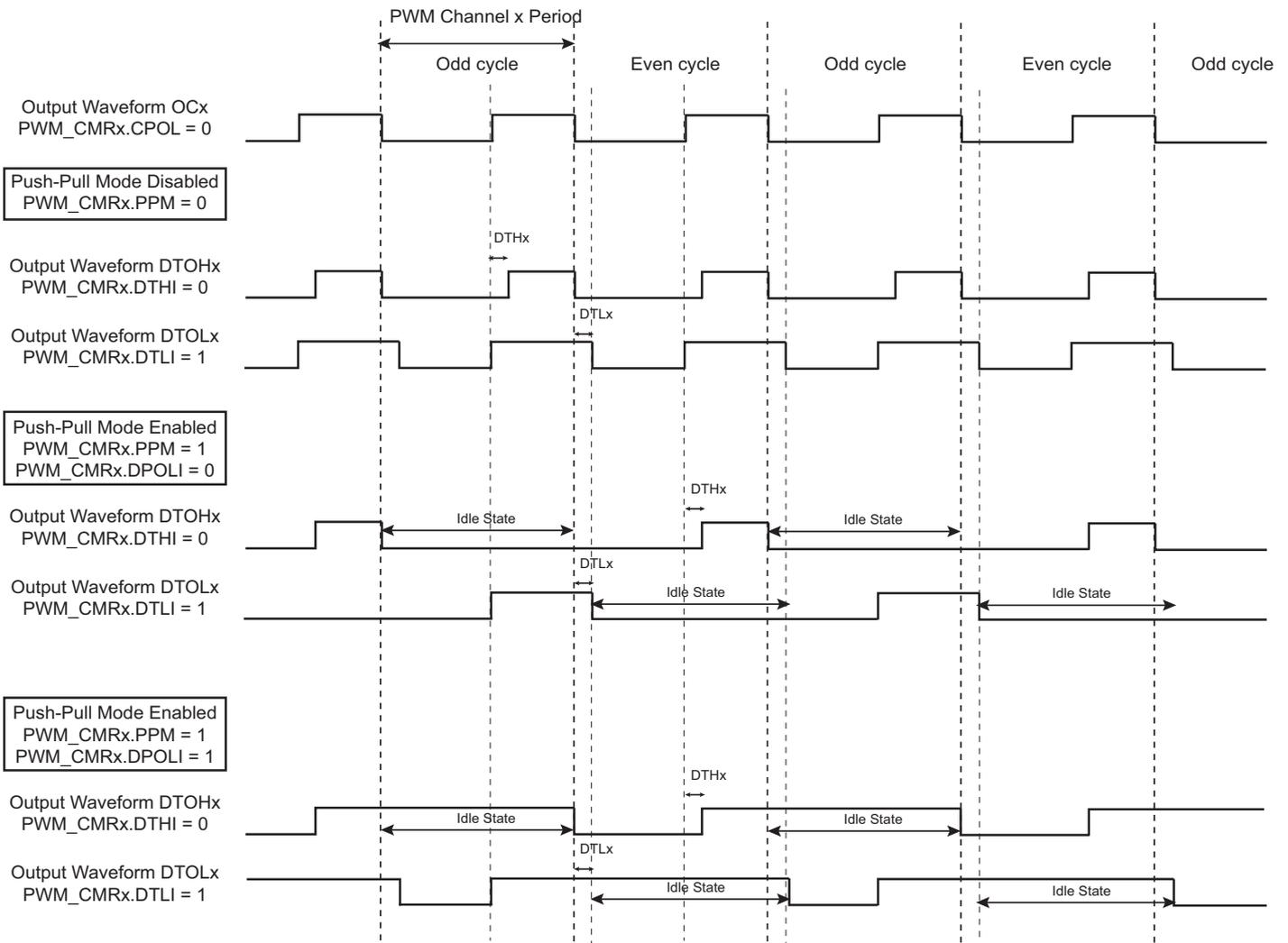
**Figure 49-11. PWM Push-Pull Waveforms: Left-Aligned Mode**
