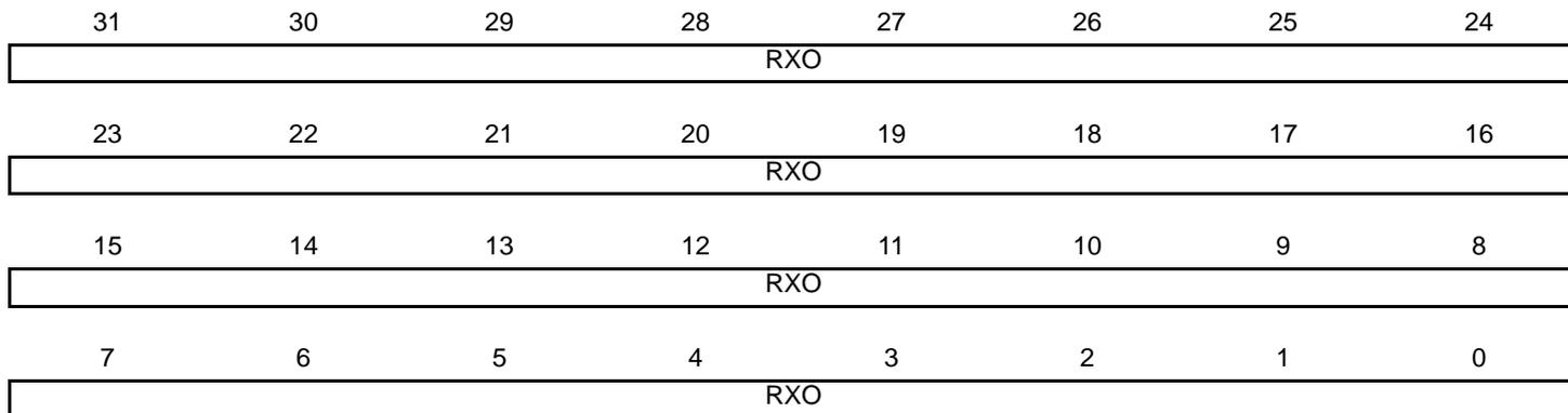
When reading the Octets Transmitted and Octets Received Registers, bits [31:0] should be read prior to bits [47:32] to ensure reliable operation.
