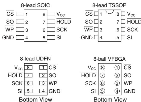
Block Write protection is enabled by programming the status register with top 1/4, top 1/2 or entire array of write protection. Separate Program Enable and Program Disable instructions are provided for additional data protection. Hardware data protection is provided via the  $\overline{WP}$  pin to protect against inadvertent write attempts to the status register. The  $\overline{HOLD}$  pin may be used to suspend any serial communication without resetting the serial sequence.
