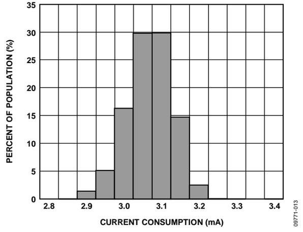
Figure 18. Current Consumption at 25°C (V<sub>RATIO</sub> = 5 V)
