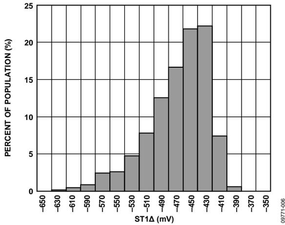
Figure 10. ST1 Output Change at 25°C ( $V_{RATIO} = 5 V$ )
