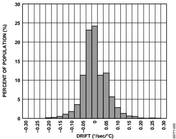
Figure 5. Null Drift over Temperature ( $V_{RATIO} = 5 V$ )
