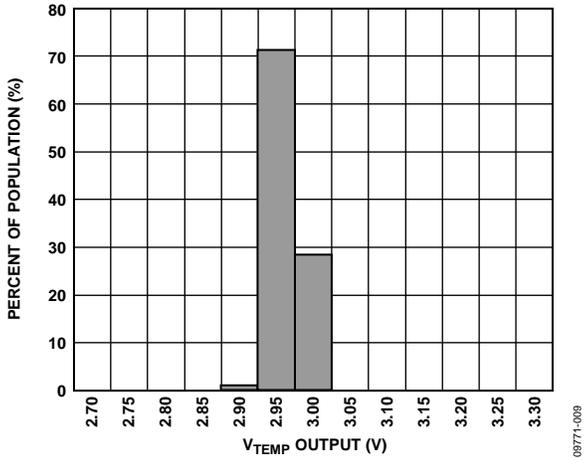
Figure 16. V<sub>TEMP</sub> Output at 25°C (V<sub>RATIO</sub> = 5 V)
