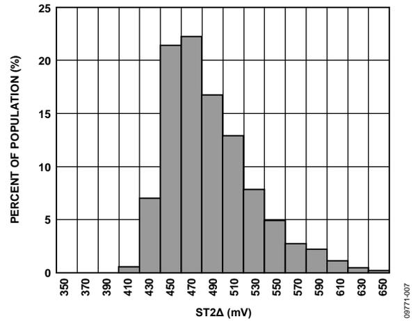
Figure 13. ST2 Output Change at 25°C ( $V_{RATIO} = 5 V$ )
