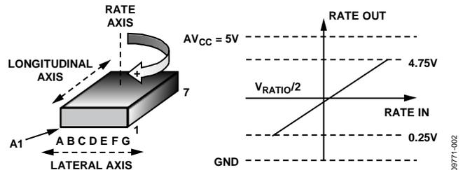
Figure 2. RATEOUT Signal Increases with Clockwise Rotation
