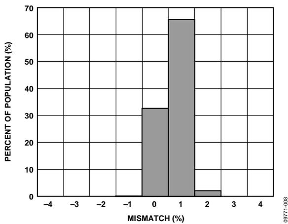
Figure 12. Self-Test Mismatch at 25°C ( $V_{RATIO} = 5 V$ )
