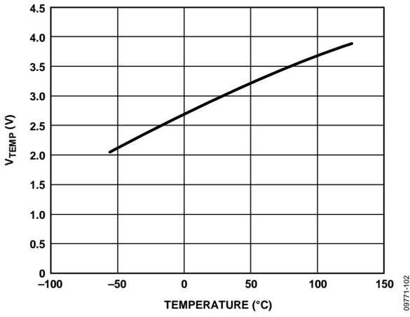
Figure 17. V<sub>TEMP</sub> Output vs. Temperature
