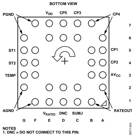
Figure 3. Pin Configuration
