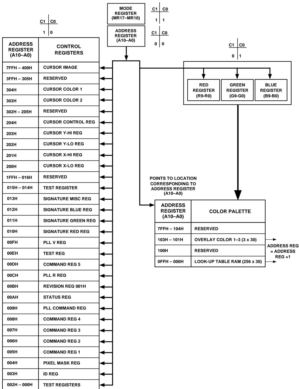
Figure 34. Internal Register Configuration and Address Decoding
