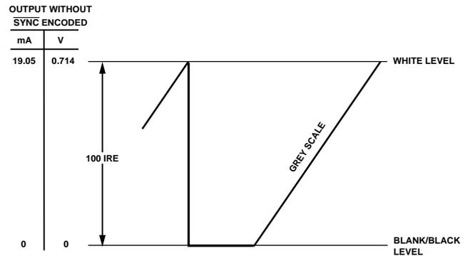
*Figure 50. Composite Video Waveform Pedestal = 0 IRE; DAC Gain = 4311*
