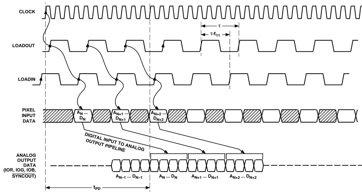
Figure 8. Pixel Input to Analog Output Pipeline with Maximum LOADOUT to LOADIN Delay (4:1 Multiplex Mode)
