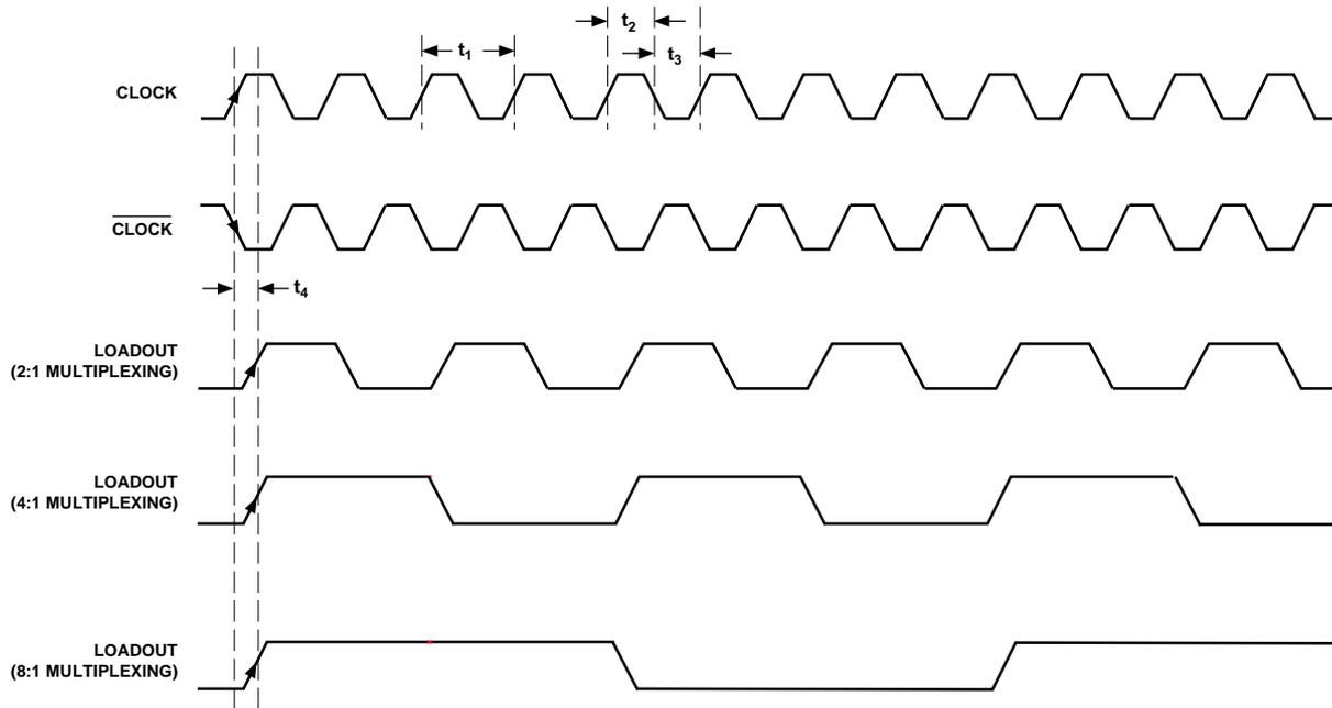
Figure 3. LOADOUT vs. Pixel Clock Input (CLOCK,  $\overline{\text{CLOCK}}$ )
