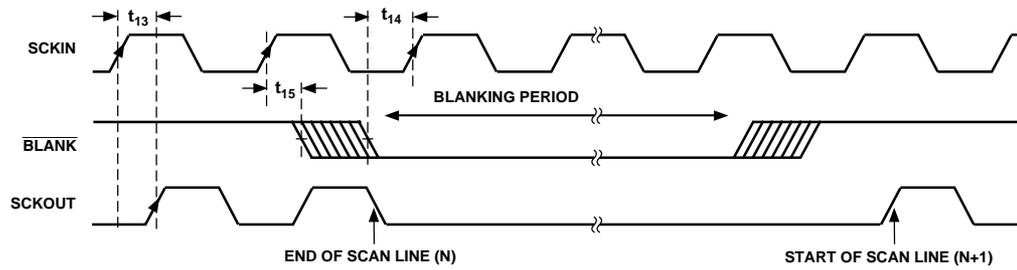
Figure 12. Video Data Shift Clock Input (SCKIN) & BLANK vs. Video Data Shift Clock Output (SCKOUT)
