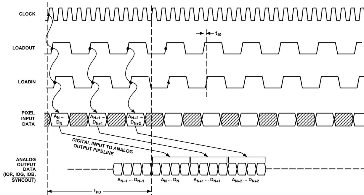
Figure 7. Pixel Input to Analog Output Pipeline with Minimum LOADOUT to LOADIN Delay (4:1 Multiplex Mode)
