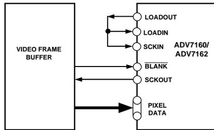
Figure 19. ADV7160/ADV7162 Interface Using SCKIN and SCKOUT
