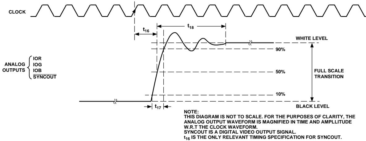
Figure 13. Analog Output Response vs. CLOCK
