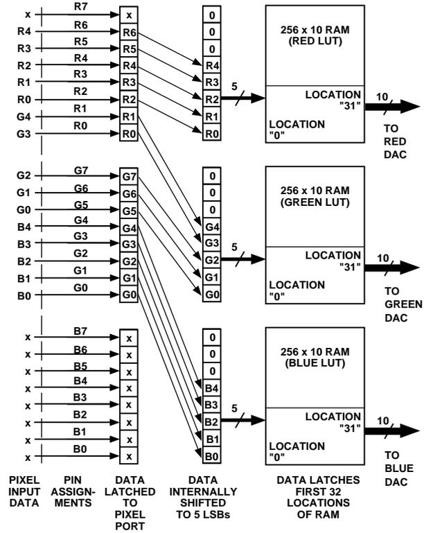
Figure 28. 15-Bit True-Color Mapping using R6-R0 and G7-G0
