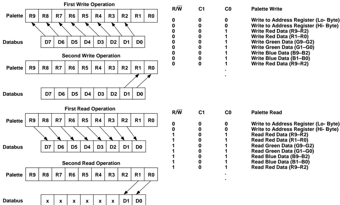
Figure 35. 8-Bit Data Bus Using 10-Bit DACs
