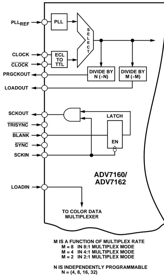
Figure 16. Clock Control Circuit of the ADV7160/ADV7162
