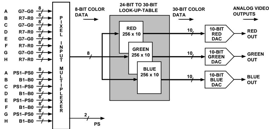
Figure 32. 8-Bit Pseudo Color in 8:1 Multiplexing Mode
