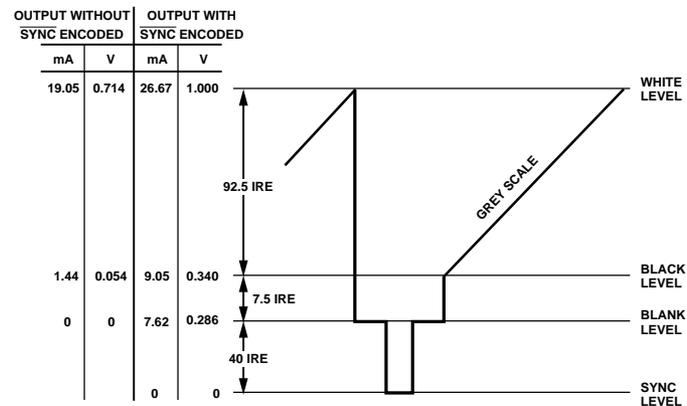
Figure 47. Composite Video Waveform SYNC Decoded; Pedestal = 7.5 IRE; DAC Gain = 3996
