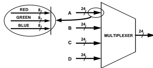
Figure 15. Multiplexed Color Inputs for the ADV7160/ADV7162
