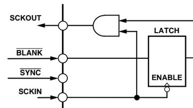
Figure 18. SCKOUT Generation Circuit
