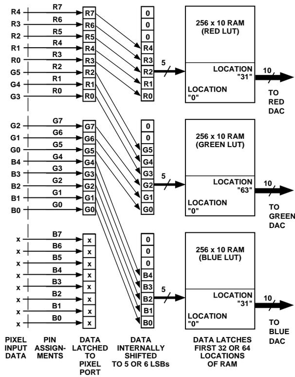
Figure 26. 16-Bit True-Color Mapping using R7-R0 and G7-G0
