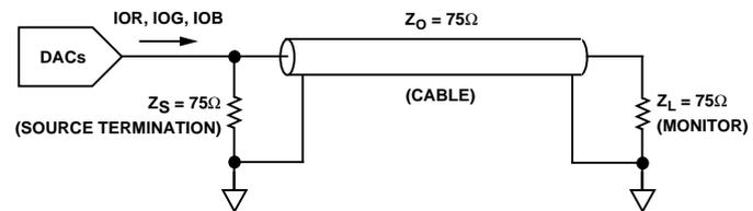
Figure 46. DAC Output Termination (Doubly Terminated  $75 \Omega$  Load)
