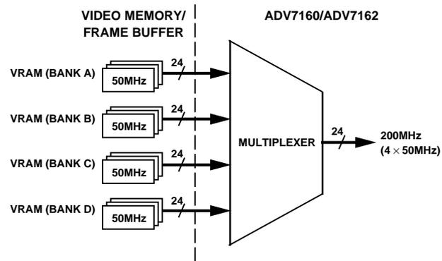
Figure 31. Direct Interfacing of Video Memory to ADV7160/ADV7162
