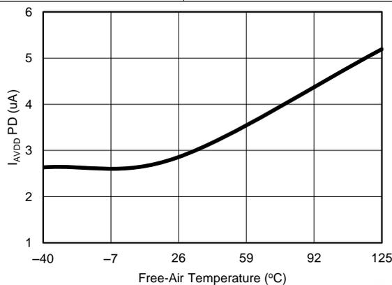
Figure 66. AVDD Current vs Temperature (Power Down)
