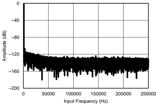
Number of points = 64k,  $f_{IN} = 1\text{ kHz}$ , SNR = 77.55 dB, SINAD = 77.5 dB, THD = -100 dB, SFDR = 107 dB
