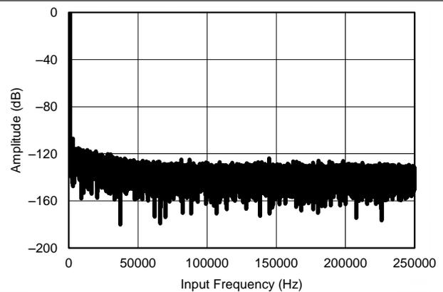
Number of points = 64k,  $f_{IN} = 1\text{ kHz}$ , SNR = 83.55 dB, SINAD = 83.5 dB, THD = -103 dB, SFDR = 107 dB
