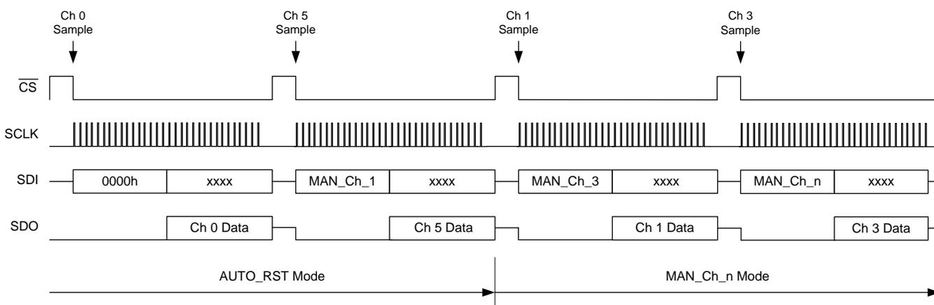
**Figure 104. Transitioning from AUTO\_RST to MAN\_Ch\_n Mode
