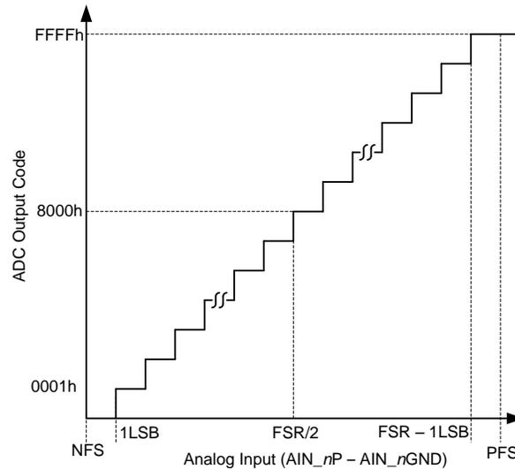
Figure 85. 16-Bit ADC Transfer Function (Straight-Binary Format)
