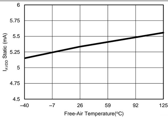
Figure 64. AVDD Current vs Temperature for the ADS8684A (During Sampling)
