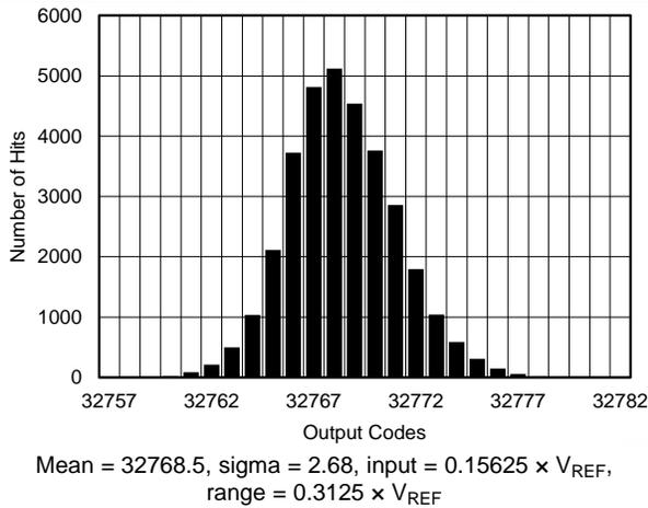
**Figure 14. DC Histogram for Mid-Scale Inputs ( $0.3125 \times V_{REF}$ )**
