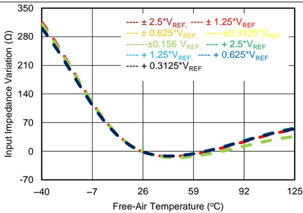
Figure 4. Input Impedance Variation vs Temperature
