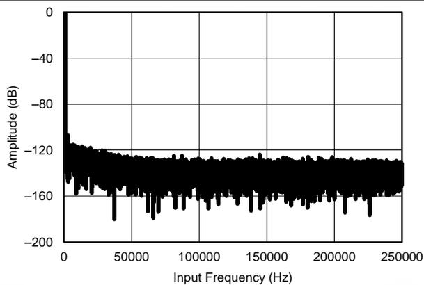
Number of points = 64k,  $f_{IN} = 1\text{ kHz}$ , SNR = 77.6 dB, SINAD = 77.6 dB, THD = -106 dB, SFDR = 107 dB
