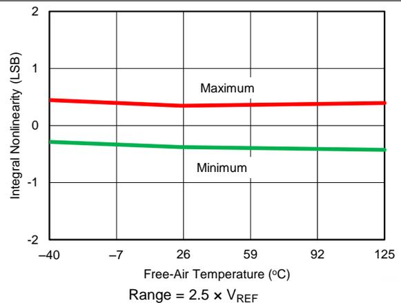
Figure 29. INL vs Temperature ( $2.5 \times V_{REF}$ )
