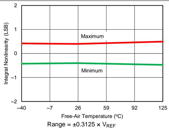
Figure 31. INL vs Temperature ( $\pm 0.3125 \times V_{REF}$ )
