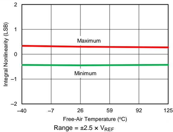
Figure 26. INL vs Temperature ( $\pm 2.5 \times V_{REF}$ )
