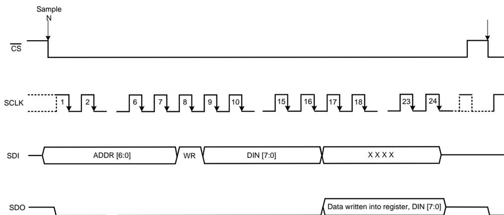
Figure 107. Program Register Write Cycle Timing Diagram
