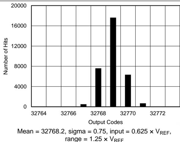
Figure 10. DC Histogram for Mid-Scale Inputs ( $1.25 \times V_{REF}$ )
