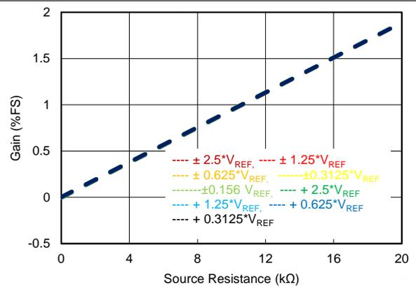
Figure 41. Gain Error vs External Resistance ( $R_{EXT}$ )
