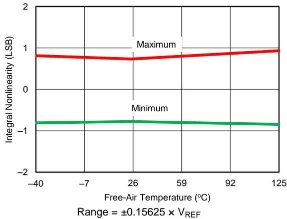
Figure 32. INL vs Temperature ( $\pm 0.15625 \times V_{REF}$ )
