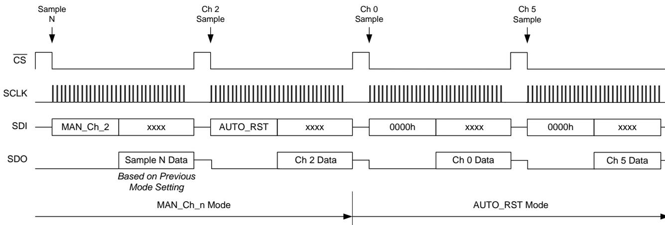
**Figure 105. Transitioning from MAN\_Ch\_n to AUTO\_RST Mode
