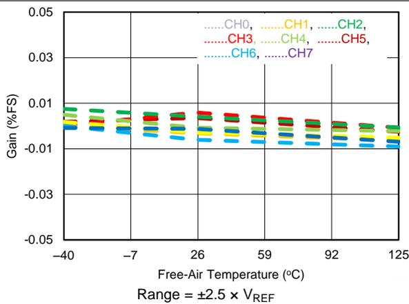
Figure 40. Gain Error vs Temperature Across Channels
