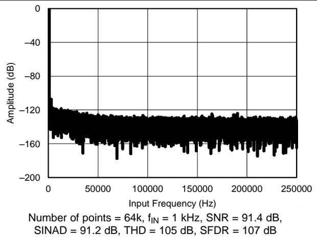
Figure 43. Typical FFT Plot ( $\pm 1.25 \times V_{REF}$ )
