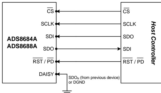
Figure 89. Pin Configuration for the Digital Interface
