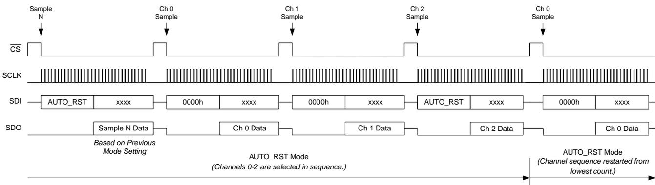
Figure 101. Device Operation Example in AUTO\_RST Mode
