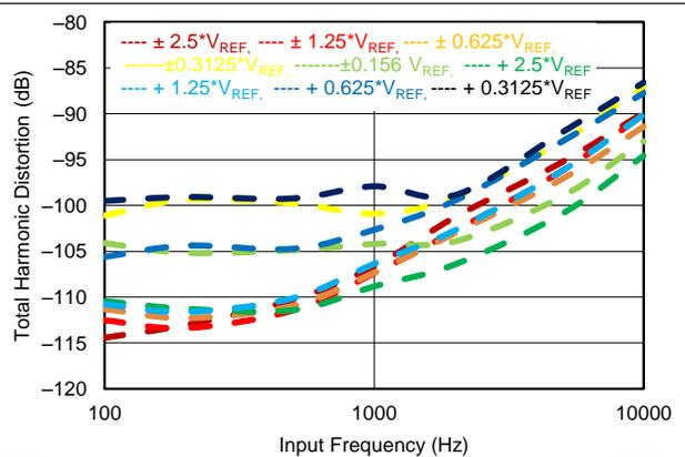
Figure 55. THD vs Input Frequency
