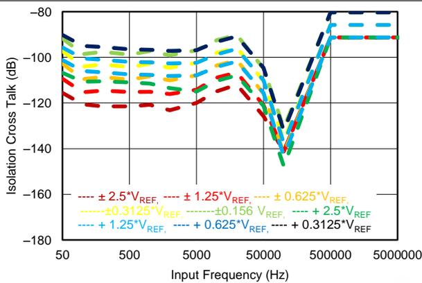
Figure 58. Isolation Crosstalk vs Frequency
