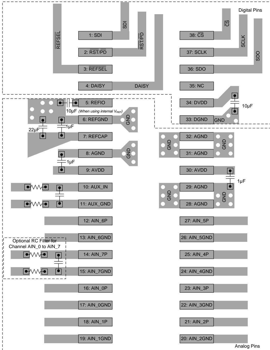
Figure 128. Board Layout for the ADS8684A and ADS8688A
