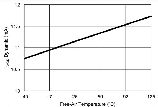
Figure 61. AVDD Current vs Temperature for the ADS8688A ( $f_S = 500\text{ kSPS}$ )
