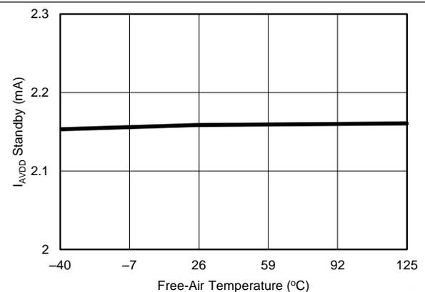
Figure 65. AVDD Current vs Temperature (STANDBY)
