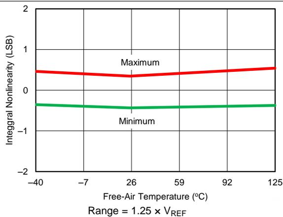
Figure 30. INL vs Temperature ( $1.25 \times V_{REF}$ )
