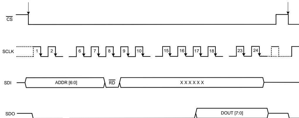
**Figure 108. Program Register Read Cycle Timing Diagram**
