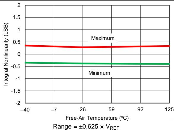
Figure 28. INL vs Temperature ( $\pm 0.625 \times V_{REF}$ )
