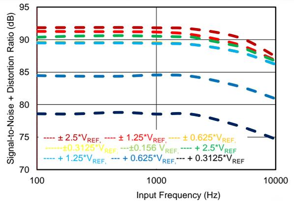
Figure 53. SINAD vs Input Frequency
