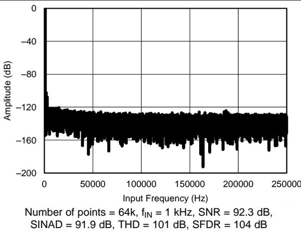
Figure 42. Typical FFT Plot ( $\pm 2.5 \times V_{REF}$ )
