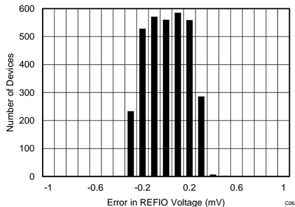
Figure 74. Internal Reference Accuracy at Room Temperature Histogram
