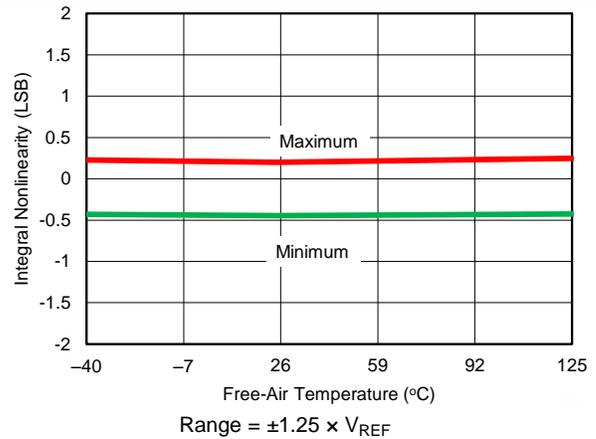
Figure 27. INL vs Temperature ( $\pm 1.25 \times V_{REF}$ )
