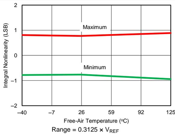
Figure 34. INL vs Temperature ( $0.3125 \times V_{REF}$ )
