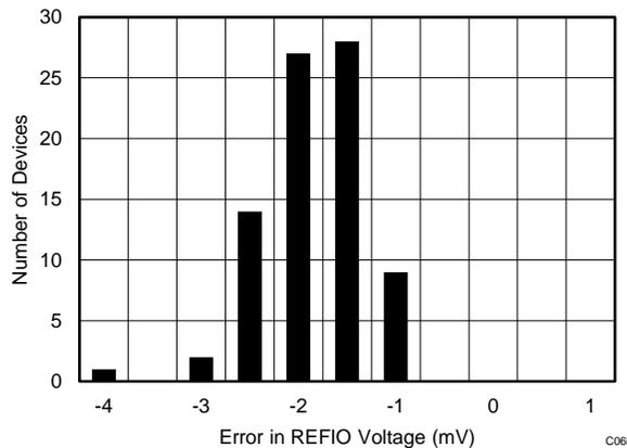
Figure 75. Solder Heat Shift Distribution Histogram
