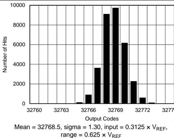
Figure 13. DC Histogram for Mid-Scale Inputs ( $0.625 \times V_{REF}$ )
