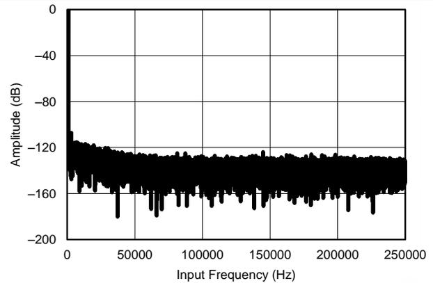
Number of points = 64k,  $f_{IN} = 1\text{ kHz}$ , SNR = 83.55 dB, SINAD = 83.5 dB, THD = -104 dB, SFDR = 107 dB
