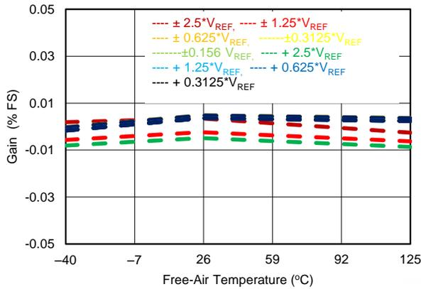
Figure 38. Gain Error vs Temperature Across Input Ranges
