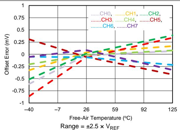
Figure 37. Offset Error vs Temperature Across Channels
