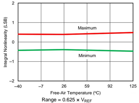
Figure 33. INL vs Temperature ( $0.625 \times V_{REF}$ )
