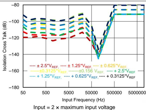
Figure 60. Isolation Crosstalk vs Frequency for Overrange Inputs
