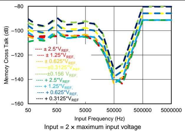
Figure 59. Memory Crosstalk vs Frequency for Overrange Inputs
