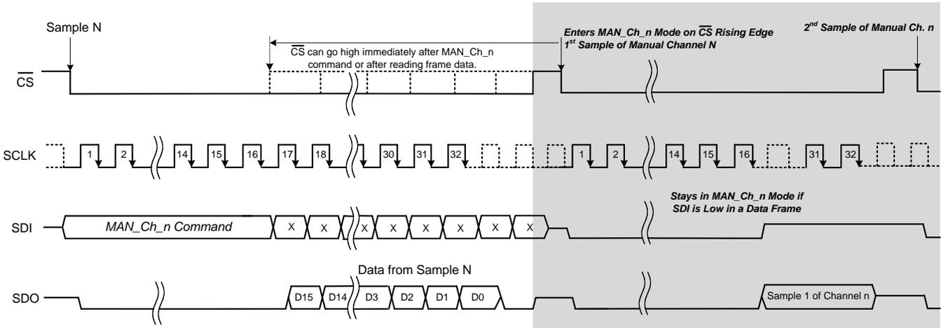
Figure 102. Enter MAN\_Ch\_n Scan Mode Timing Diagram
