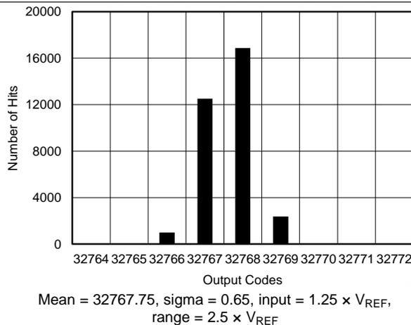
Figure 9. DC Histogram for Mid-Scale Inputs ( $2.5 \times V_{REF}$ )
