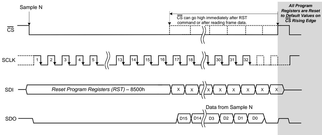
Figure 106. Reset Program Registers (RST) Timing Diagram
