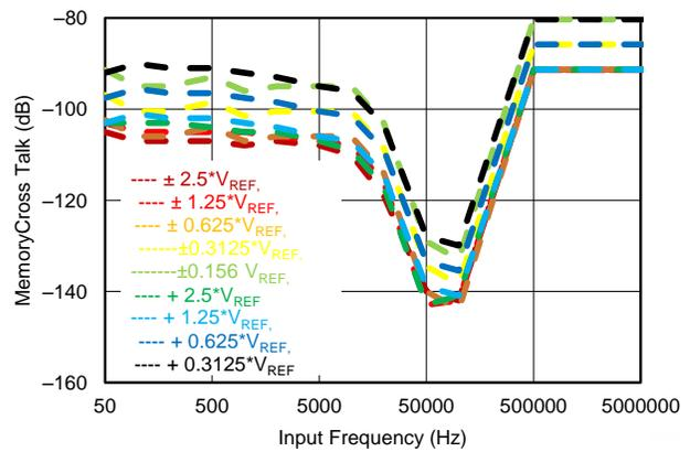
Figure 57. Memory Crosstalk vs Frequency
