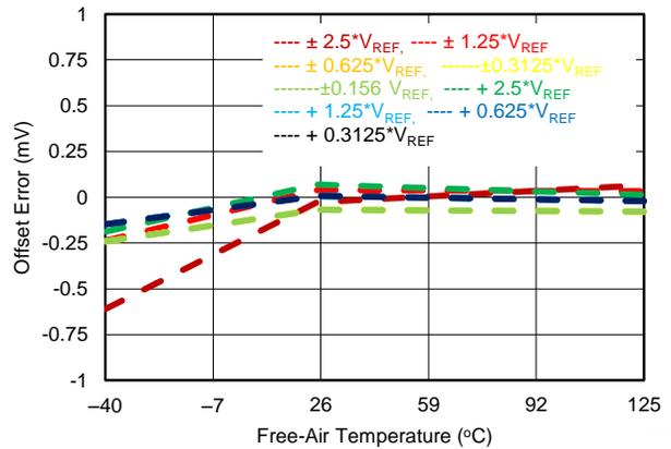
Figure 35. Offset Error vs Temperature Across Input Ranges
