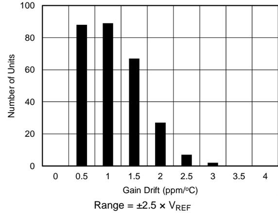
Figure 39. Typical Histogram for Gain Error Drift
