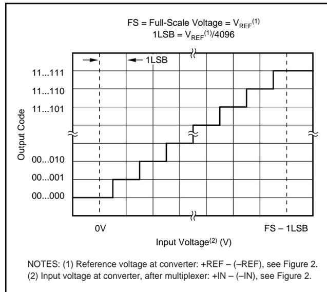
FIGURE 13. Ideal Input Voltages and Output Codes.
