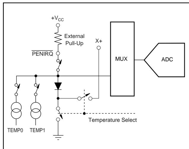
FIGURE 6. Functional Block Diagram of Temperature Measurement Mode.
