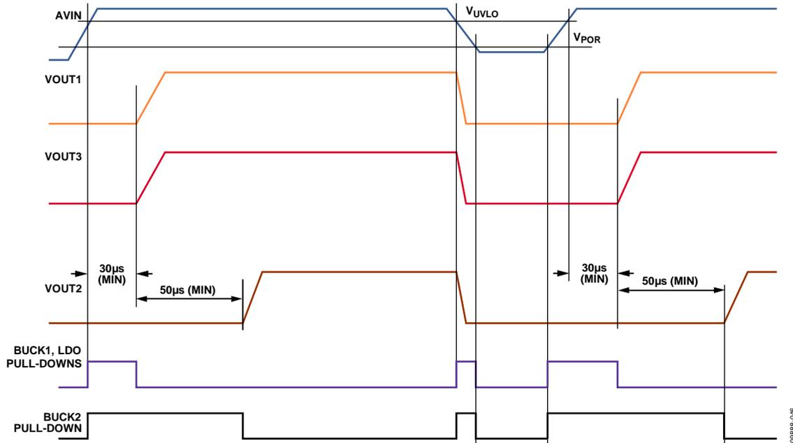
Figure 46. Regulator Sequencing (EN1 = EN2 = EN3 = VAVIN)
