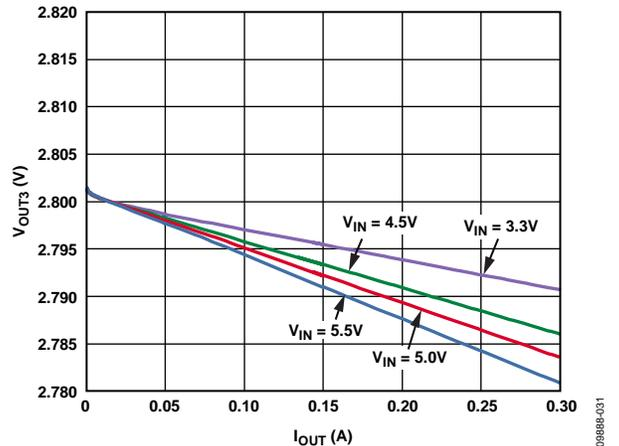
Figure 31. LDO Load Regulation Across Input Voltage,  $V_{OUT3} = 2.8$  V
