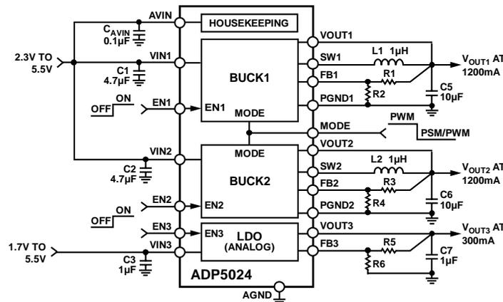
Figure 53. Adjustable Output Voltages with Enable Pins
