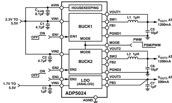
Figure 52. Fixed Output Voltages with Enable Pins
