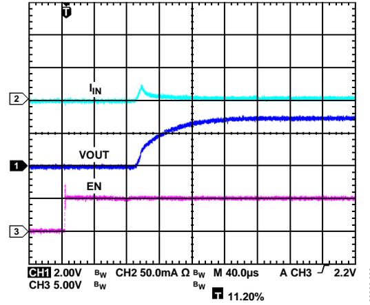
Figure 30. LDO Startup,  $V_{OUT3} = 3.0$  V,  $I_{OUT3} = 5$  mA
