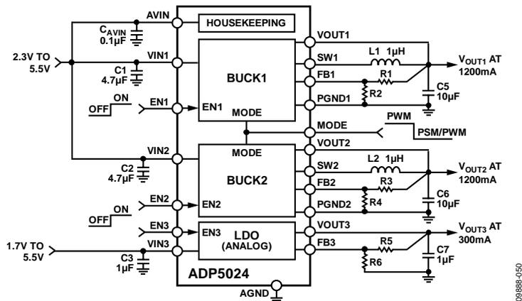
Figure 50. Processor System Power Management with PSM/PWM Control
