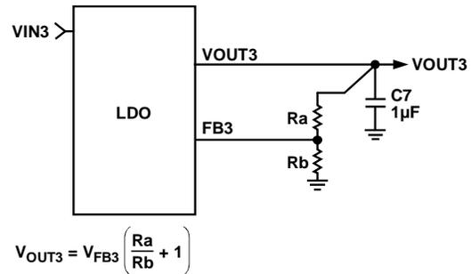
Figure 48. LDO External Output Voltage Setting
