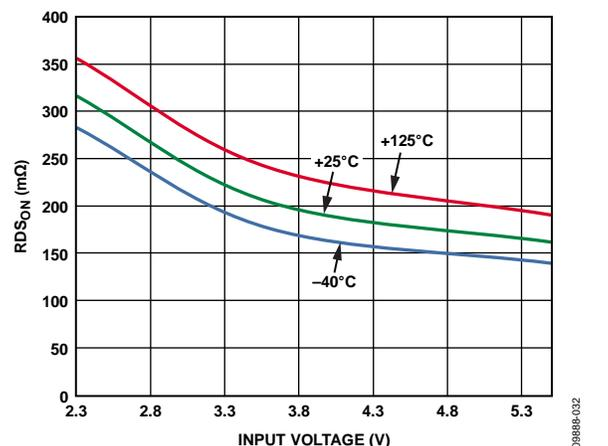
Figure 32. NMOS  $R_{DS(on)}$  vs. Input Voltage Across Temperature
