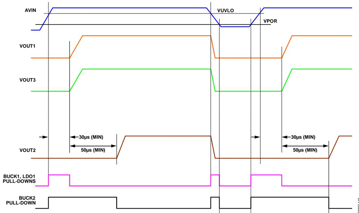
Figure 46. Regulator Sequencing on ADP5023 (EN1 = EN2 = EN3 = V<sub>AVIN</sub>)
