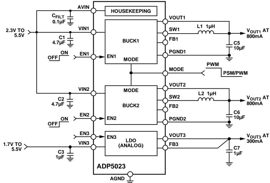
Figure 52. ADP5023 Fixed Output Voltages with Enable Pins
