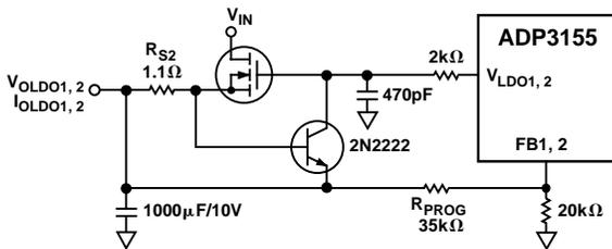
Figure 15. Linear Regulator with Overcurrent Protection
