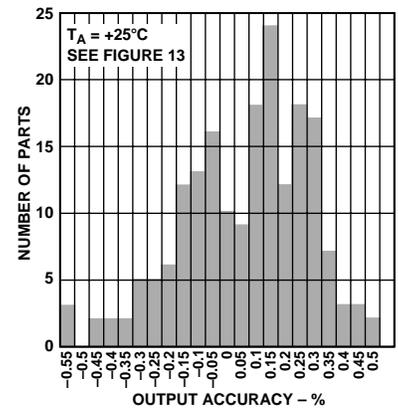
Figure 12. Output Accuracy Distribution,  $V_{OUT} = 2.0 V$
