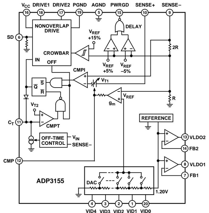
The ADP3155 contains two linear regulator controllers that are designed to drive external N-channel MOSFETs. These linear regulators are used to generate the auxiliary voltages (AGP, GTL, etc.) required in most motherboard designs, and have been designed to provide a high bandwidth load-transient response. A pair of external feedback resistors sets each linear regulator output voltage.
