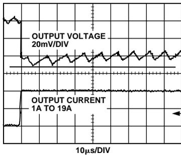
Figure 10. Transient Response, 1 A-19 A of Figure 2 Circuit
