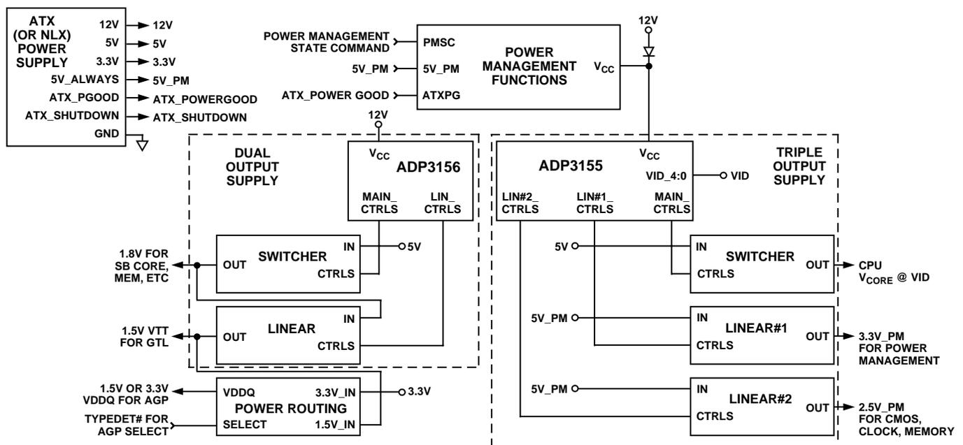
Figure 14. ACPI-Compliant Pentium III System Block Diagram
