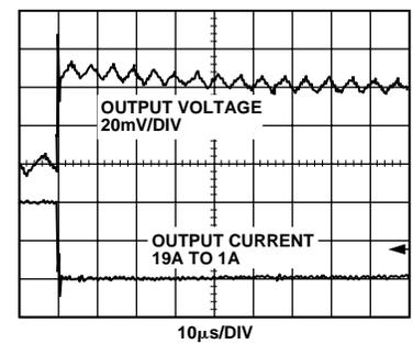
Figure 9. Transient Response, 19 A-1 A of Figure 2 Circuit
