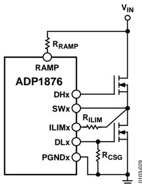
Figure 29. Slope Compensation and CS Gain Connection
