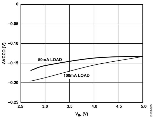
Figure 5. VCCO Dropout
