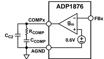
Figure 31. Compensation Components
