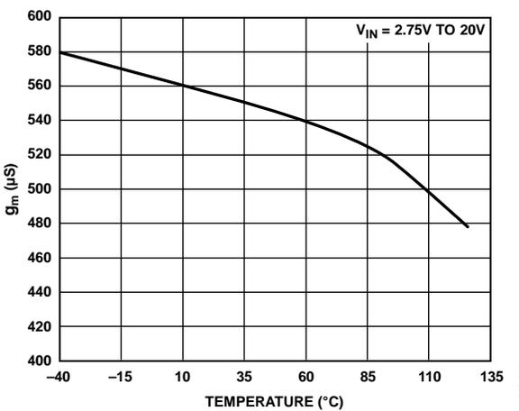
Figure 18.  $g_m$  of Error Amplifier vs. Temperature
