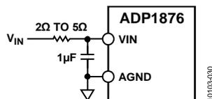
Figure 30. Input Filter Configuration
