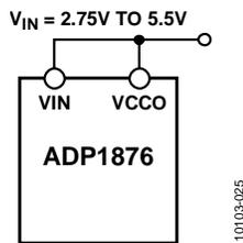
Figure 25. Configuration for  $V_{IN} < 5.5$  V
