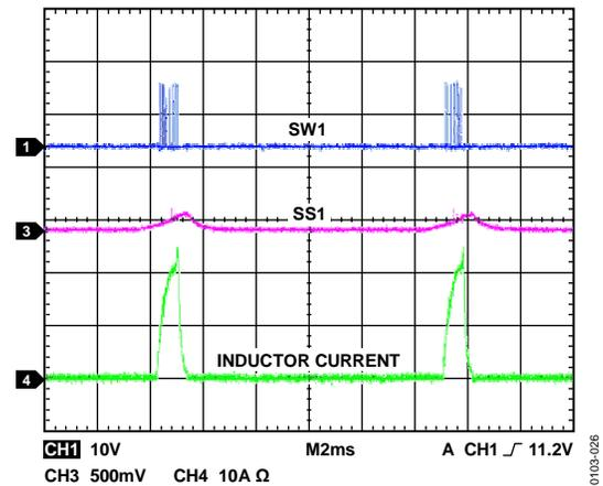
Figure 26. Current-Limit Hiccup Mode, 20 A Circuit
