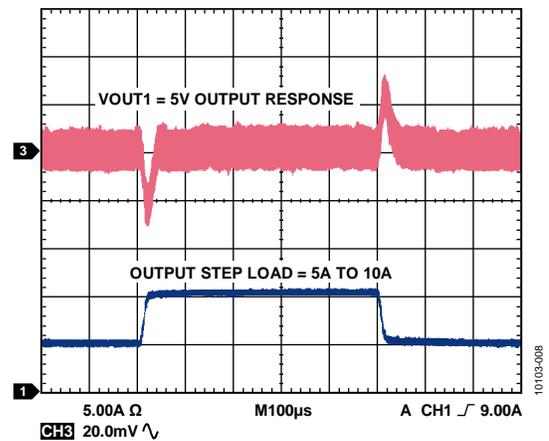
Figure 8. Step Load Transient of Figure 33
