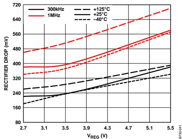
Figure 42. Internal Boost Rectifier Drop vs.  $V_{REG}$
