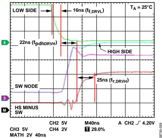
Figure 60. Upper-Side Driver Rising and Lower-Side Falling Edge Waveforms
