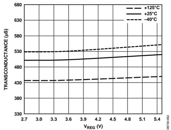
Figure 63. Transconductance ( $G_m$ ) vs.  $V_{REG}$
