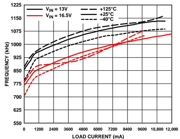
Figure 33. Frequency vs. Load Current, 1.0 MHz,  $V_{OUT} = 1.8 V$
