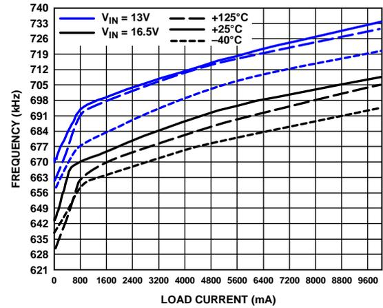
Figure 31. Frequency vs. Load Current, 600 kHz,  $V_{OUT} = 5 V$
