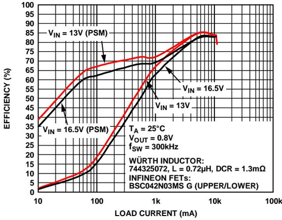
Figure 4. Efficiency—300 kHz,  $V_{OUT} = 0.8 V$
