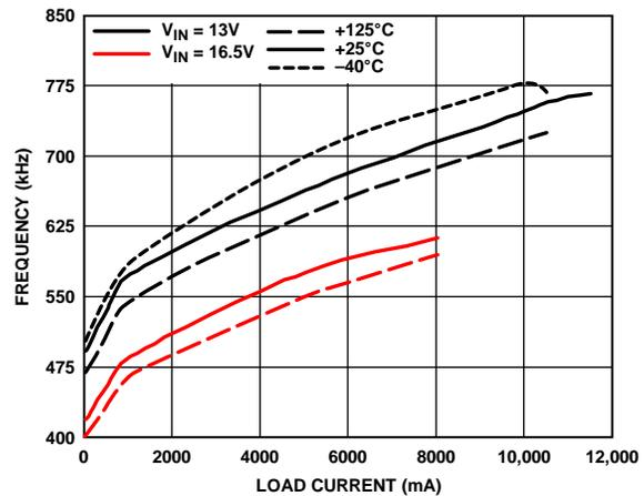
Figure 32. Frequency vs. Load Current,  $V_{OUT} = 1.0 MHz, 0.8 V$
