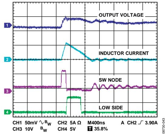
Figure 44. Power Saving Mode (PSM) Operational Waveform, 100 mA
