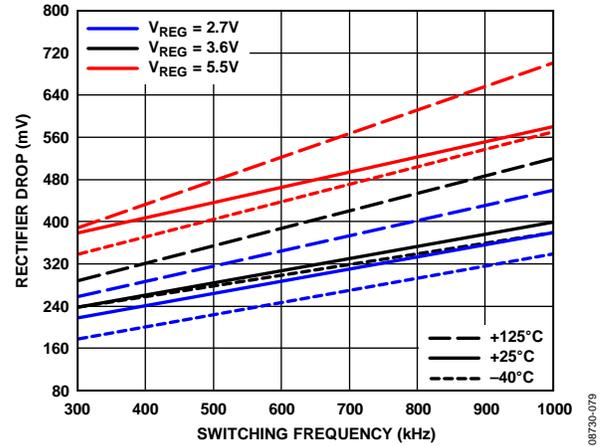
Figure 81. Internal Rectifier Voltage Drop vs. Switching Frequency
