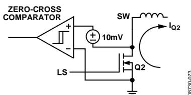
Figure 75. Zero-Cross Comparator with 10 mV of Offset
