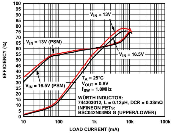
Figure 10. Efficiency—1.0 MHz,  $V_{OUT} = 0.8 V$
