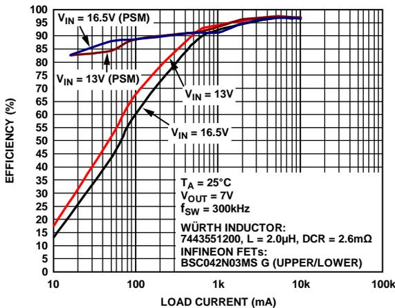
Figure 6. Efficiency—300 kHz,  $V_{OUT} = 7 V$
