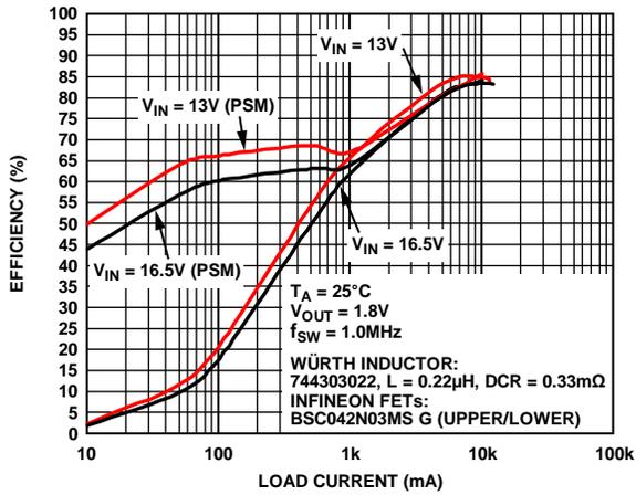
Figure 11. Efficiency—1.0 MHz,  $V_{OUT} = 1.8 V$
