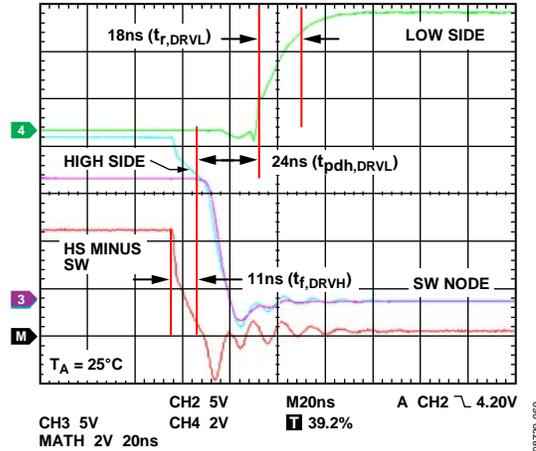
Figure 61. Upper-Side Driver Falling and Lower-Side Rising Edge Waveforms
