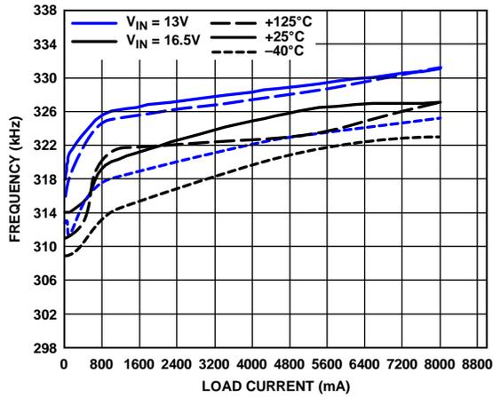
Figure 28. Frequency vs. Load Current, 300 kHz,  $V_{OUT} = 7 V$
