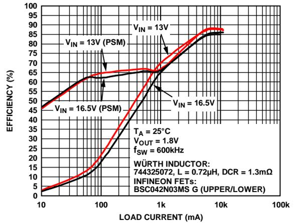
Figure 8. Efficiency—600 kHz,  $V_{OUT} = 1.8 V$
