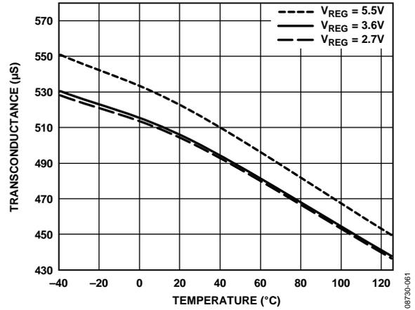
Figure 62. Transconductance ( $G_m$ ) vs. Temperature
