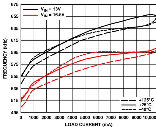
Figure 30. Frequency vs. Load Current, 600 kHz,  $V_{OUT} = 1.8 V$
