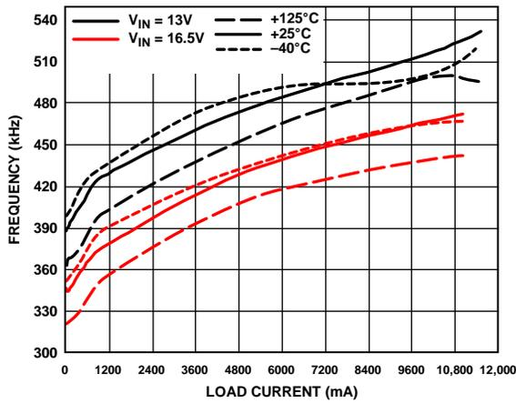
Figure 29. Frequency vs. Load Current, 600 kHz,  $V_{OUT} = 0.8 V$
