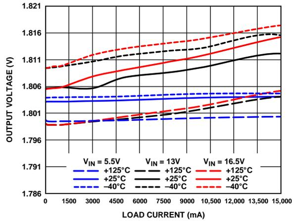
Figure 14. Output Voltage Accuracy—300 kHz,  $V_{OUT} = 1.8 V$
