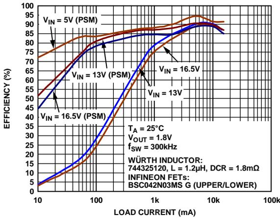
Figure 5. Efficiency—300 kHz,  $V_{OUT} = 1.8 V$
