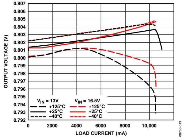
Figure 13. Output Voltage Accuracy—300 kHz,  $V_{OUT} = 0.8 V$
