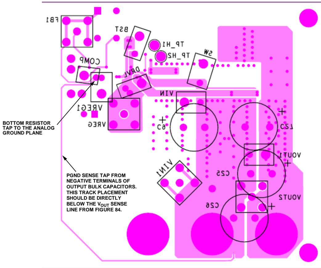
Figure 88. Layer 4 (Bottom Layer) of Evaluation Board
