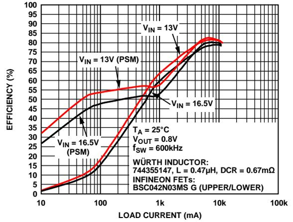
Figure 7. Efficiency—600 kHz,  $V_{OUT} = 0.8 V$
