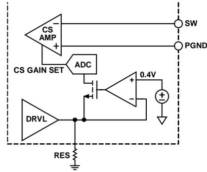
Figure 69. RES Detect Circuit for Current-Sense Gain Programming
