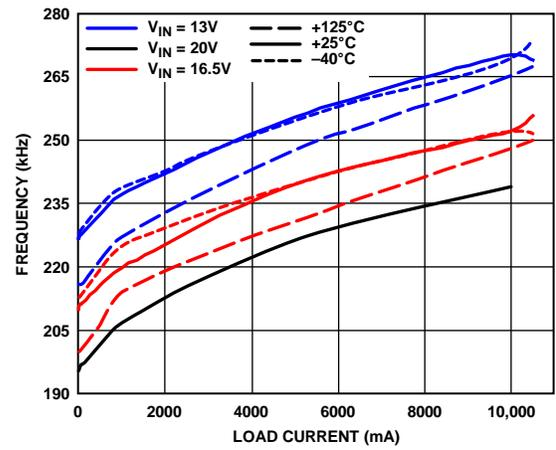
Figure 26. Frequency vs. Load Current, 300 kHz,  $V_{OUT} = 0.8$  V
