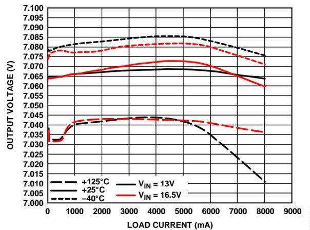
Figure 15. Output Voltage Accuracy—300 kHz,  $V_{OUT} = 7 V$
