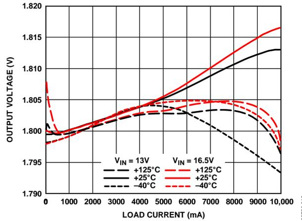
Figure 20. Output Voltage Accuracy—1.0 MHz,  $V_{OUT} = 1.8\text{ V}$
