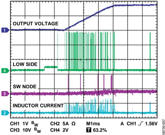
Figure 58. Soft Start and RES Detect Waveform
