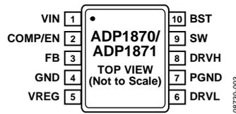
Figure 3. Pin Configuration
