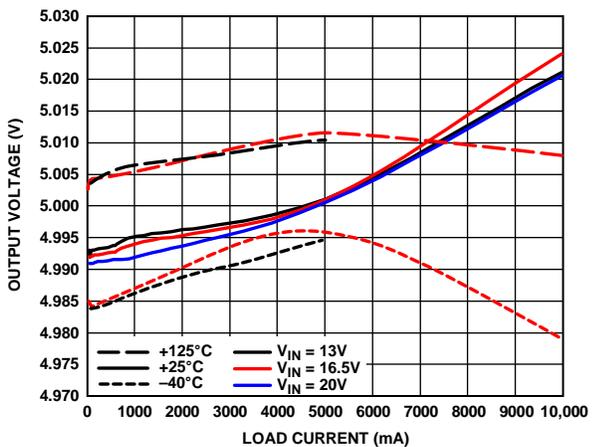
Figure 18. Output Voltage Accuracy—600 kHz,  $V_{OUT} = 5\text{ V}$
