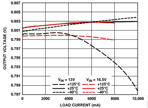
Figure 19. Output Voltage Accuracy—1.0 MHz,  $V_{OUT} = 0.8\text{ V}$
