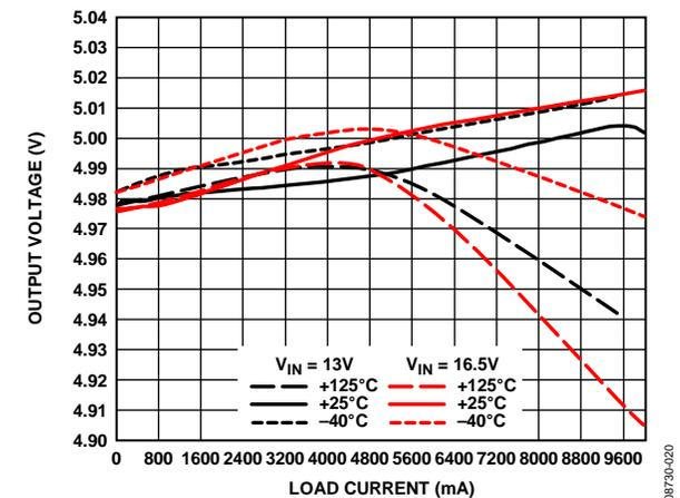
Figure 21. Output Voltage Accuracy—1.0 MHz,  $V_{OUT} = 5\text{ V}$
