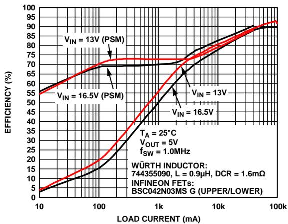
Figure 12. Efficiency—1.0 MHz,  $V_{OUT} = 5 V$
