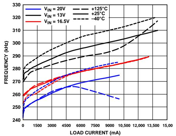
Figure 27. Frequency vs. Load Current, 300 kHz,  $V_{OUT} = 1.8$  V
