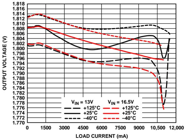
Figure 17. Output Voltage Accuracy—600 kHz,  $V_{OUT} = 1.8\text{ V}$
