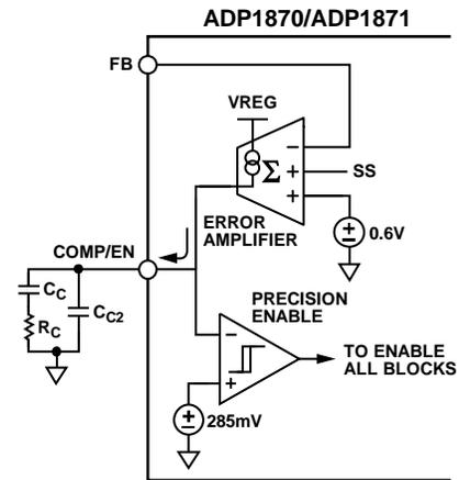
Figure 66. Release COMP/EN Pin to Enable the ADP1870/ADP1871
