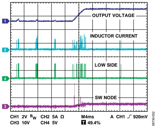
Figure 53. Output Short-Circuit Behavior Leading to Hiccup Mode
