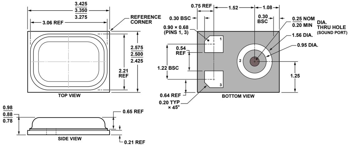
Figure 11. 3-Terminal Chip Array Small Outline No Lead Cavity [LGA\_CAV]
