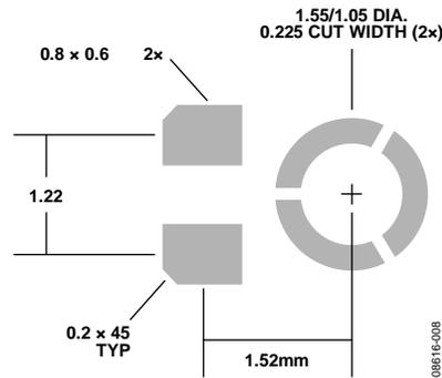
Figure 10. Suggested Solder Paste Stencil Pattern Layout
