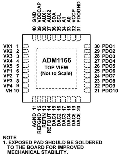
Figure 3. 40-Lead LFCSP Pin Configuration
