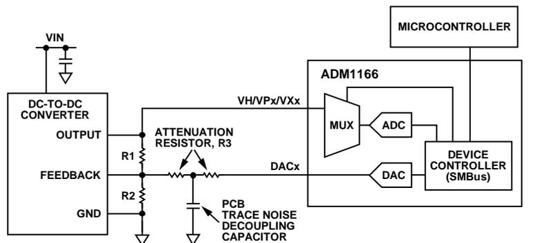
Figure 33. Closed-Loop Margining System Using the ADM1166
