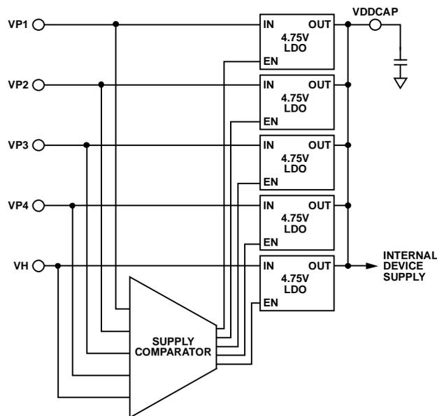
Figure 21.  $V_{DD}$  Arbitrator Operation
