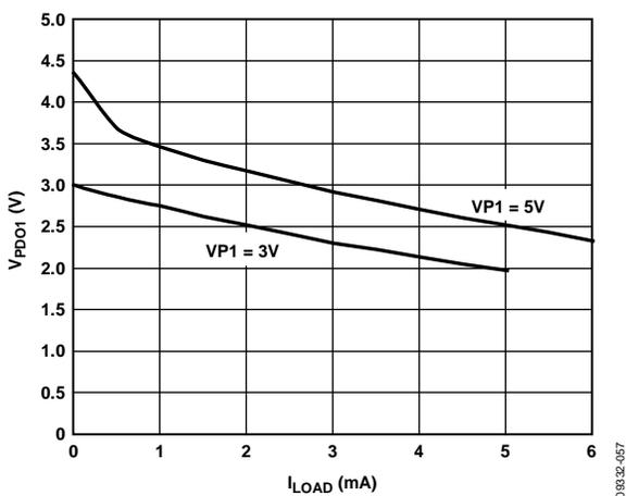
Figure 12.  $V_{PDO1}$  (Strong Pull-Up to  $VPx$ ) vs.  $I_{LOAD}$
