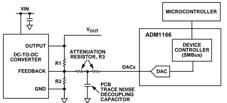
Figure 32. Open-Loop Margining System Using the ADM1166
