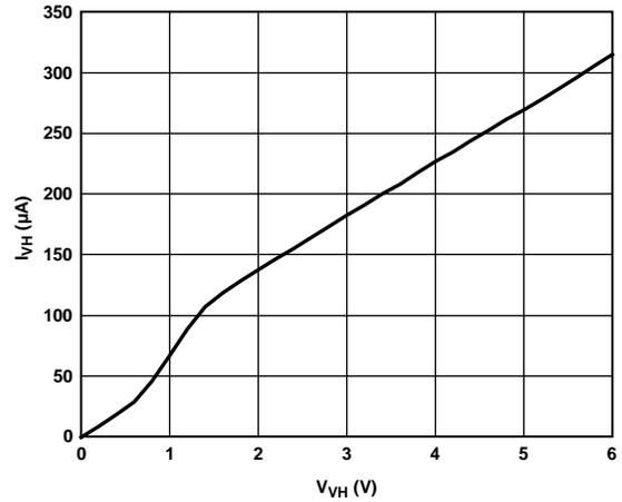
Figure 10.  $I_{VH}$  vs.  $V_{VH}$  (VH Not as Supply)
