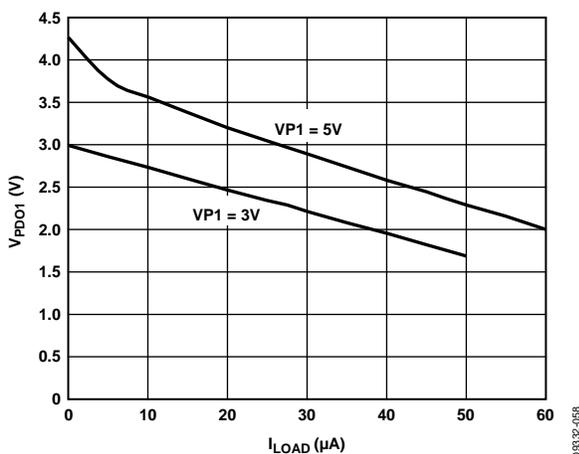
Figure 13.  $V_{PDO1}$  (Weak Pull-Up to  $VPx$ ) vs.  $I_{LOAD}$
