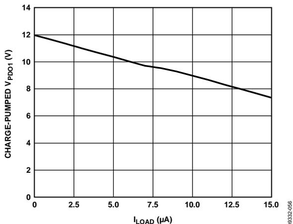
Figure 11. Charge-Pumped  $V_{PDO1}$  (FET Drive Mode) vs.  $I_{LOAD}$
