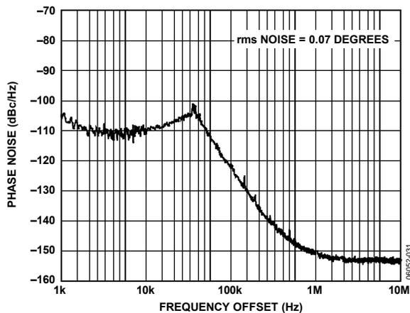
Figure 7. Integrated Phase Noise (400 MHz, 1 MHz, 50 kHz)
