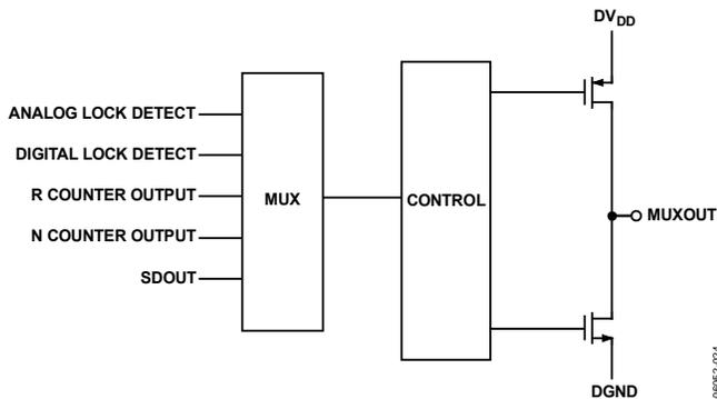
Figure 15. MUXOUT Circuit
