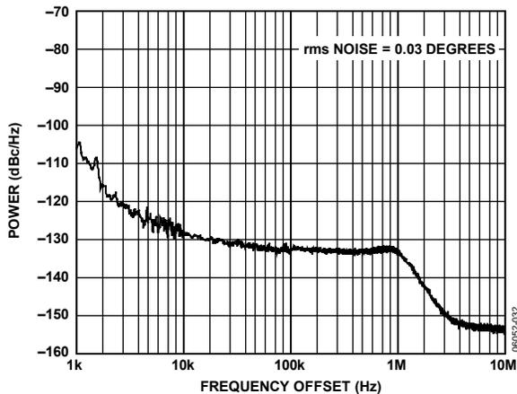
Figure 8. Integrated Phase Noise (400 MHz, PFD = 200 MHz, 50 kHz)
