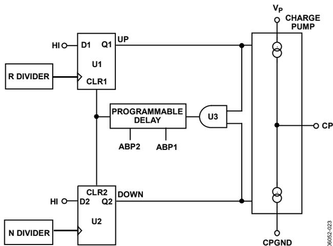
Figure 14. PFD Simplified Schematic and Timing (In Lock)
