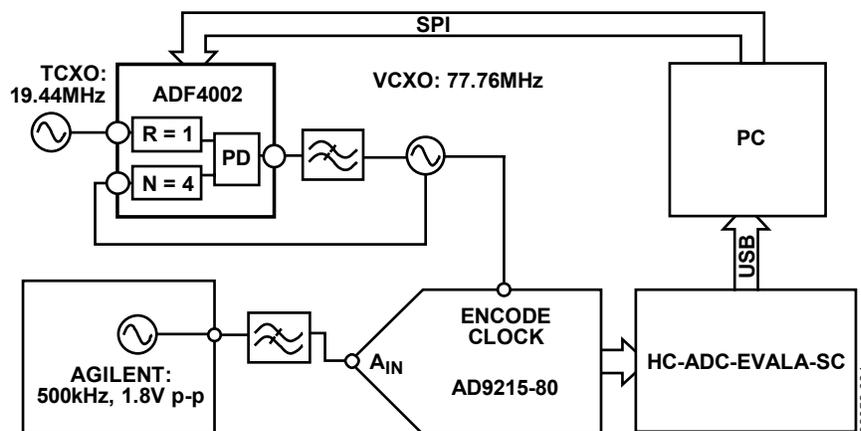
Figure 21. ADF4002 as Encode Clock
