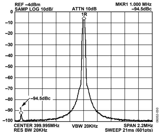
Figure 10. Reference Spurs (400 MHz, 1 MHz, 7 kHz)
