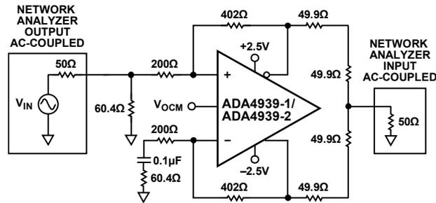
Figure 40. Test Circuit for Output Balance, CMRR
