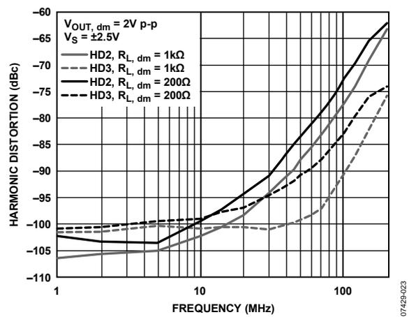
Figure 18. Harmonic Distortion vs. Frequency at Various Loads
