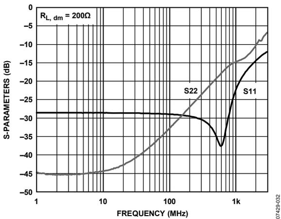
Figure 27. Return Loss (S11, S22) vs. Frequency
