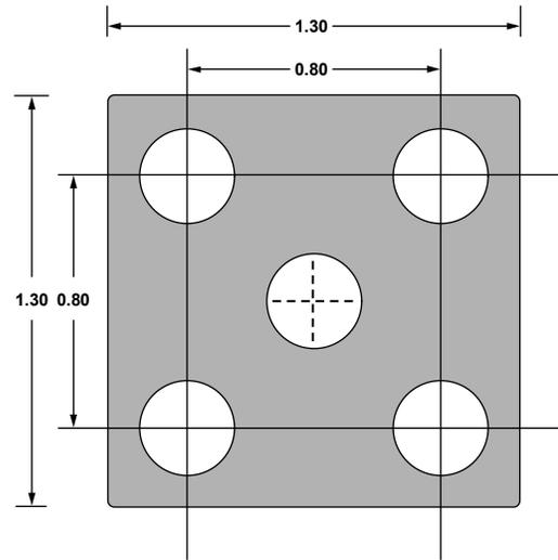
Figure 52. Recommended PCB Thermal Attach Pad Dimensions (Millimeters)
