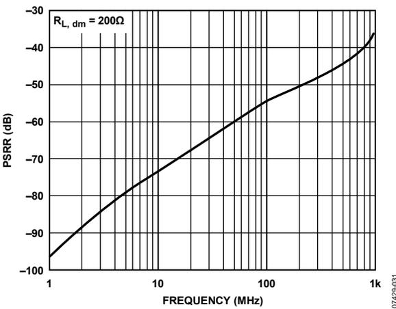
Figure 26. PSRR vs. Frequency,  $R_L = 200\ \Omega$
