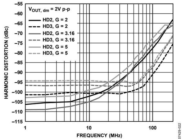
Figure 17. Harmonic Distortion vs. Frequency at Various Gains
