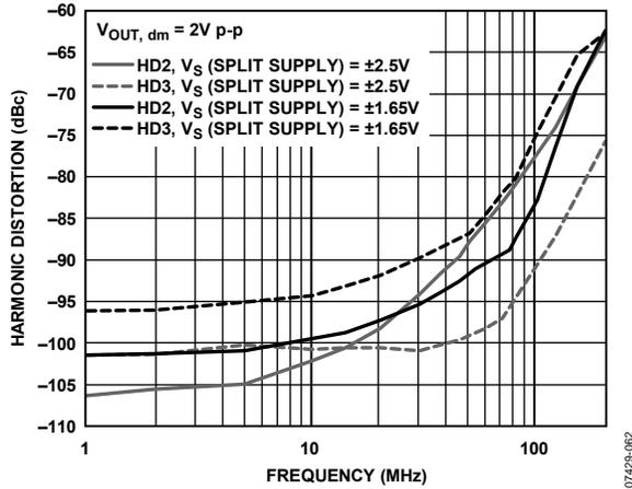
Figure 19. Harmonic Distortion vs. Frequency at Various Supplies
