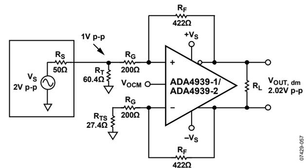
Figure 50. Terminated Single-Ended-to-Differential System with  $G = 2$
