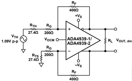
Figure 49. Thevenin Equivalent and Matched Gain Resistors
