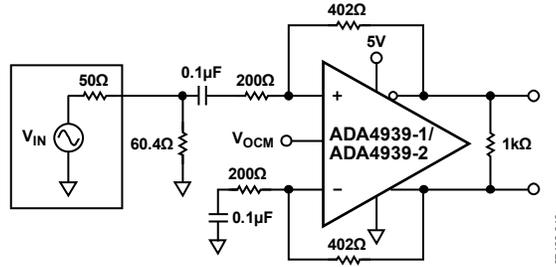
Figure 39. Equivalent Basic Test Circuit,  $G = 2$
