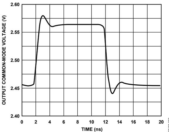
Figure 33.  $V_{OCM}$  Small Signal Pulse Response
