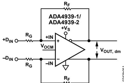
Figure 44. ADA4939-1/ADA4939-2 Configured for Balanced (Differential) Inputs
