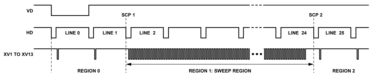
Figure 48. Example of Sweep Region for High Speed Vertical Shift
