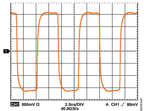
Figure 14. Output Waveform (Differential), HSTL at 16 mA, 122.88 MHz
