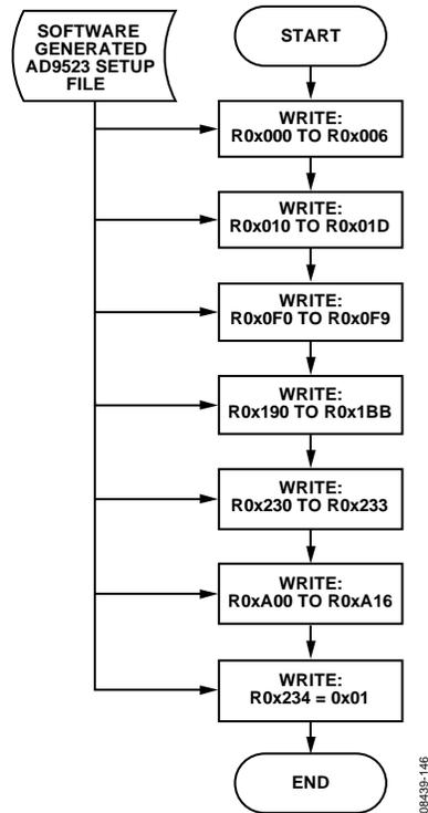
Figure 45. Subprocess: Write Registers from Setup File
