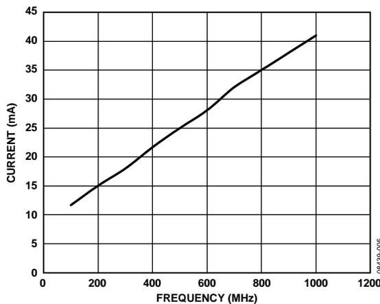
Figure 5. VDD3\_OUT[x:y] Current (Typical) vs. Frequency, LVPECL Mode
