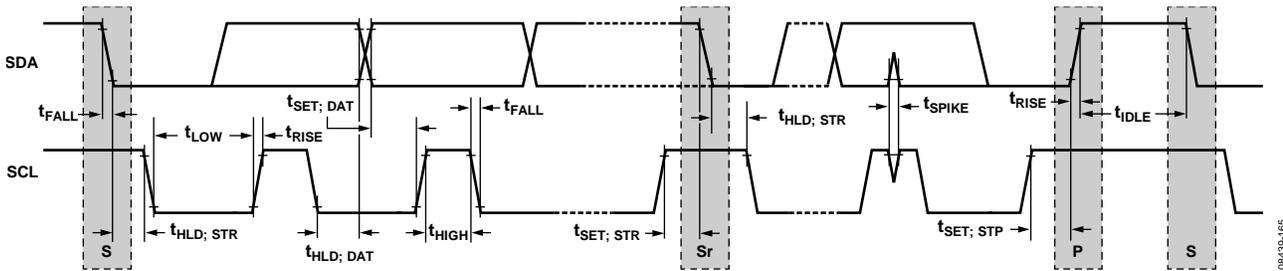
Figure 34. I<sup>2</sup>C Serial Port Timing
