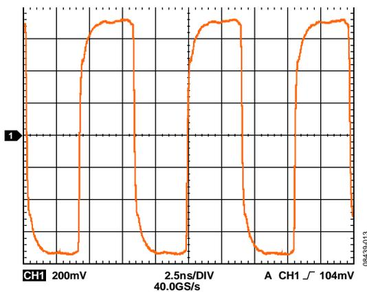
Figure 11. Output Waveform (Differential), LVPECL at 122.88 MHz
