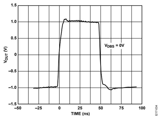
Figure 33. Full-Scale Transient Response, V<sub>DBS</sub> = 0V
