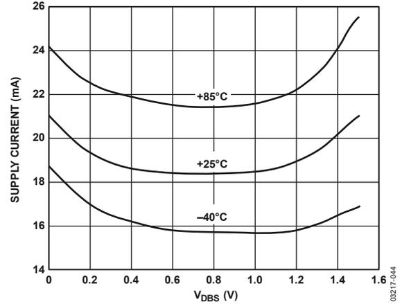
Figure 43. Supply Current vs.  $V_{DBS}$  at Three Temperatures
