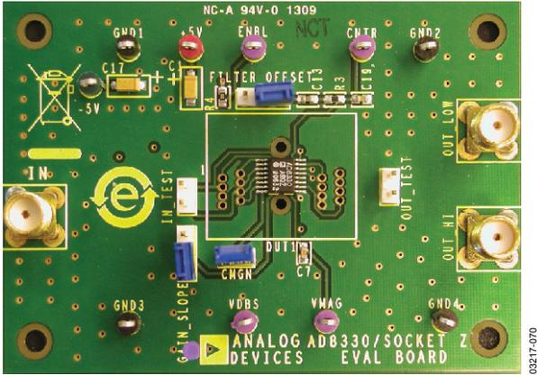
Figure 69. Photograph of the **AD8330** Evaluation Board
