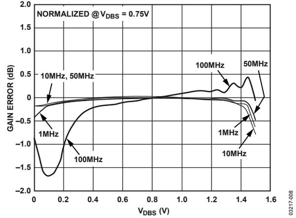
Figure 7. Gain Error vs.  $V_{DBS}$  at Various Frequencies
