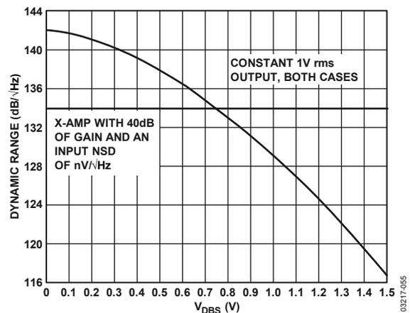
Figure 54. Dynamic Range in dB/√Hz vs. V<sub>DBS</sub> (V<sub>MAG</sub> = 0.5 V, 1 V rms Output) Compared with a Representative X-AMP (Simulation)
