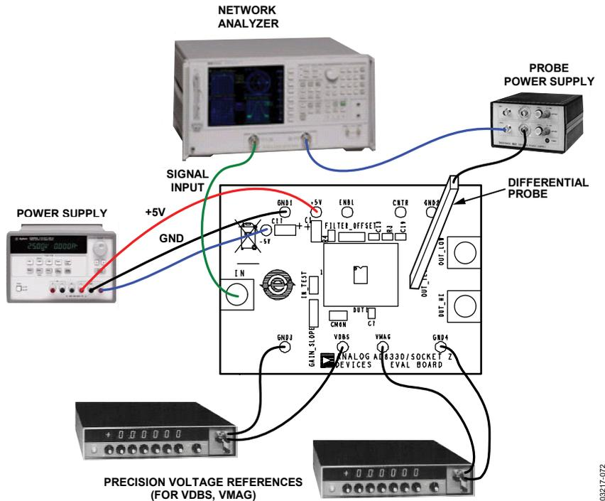
Figure 71. Typical Connections
