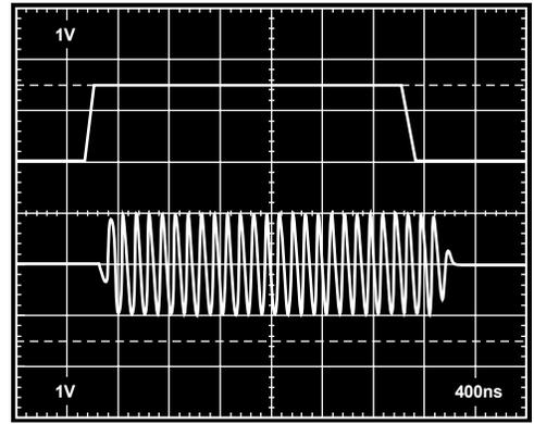
Figure 37.  $V_{DBS}$  Interface Response, Top:  $V_{DBS}$ , Bottom:  $V_{OUT}$
