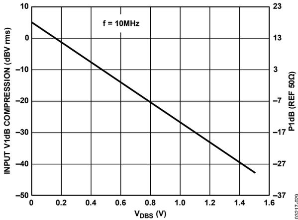
Figure 28. Input V1dB Compression vs. V<sub>DBS</sub>
