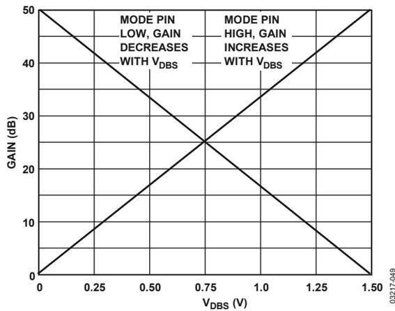
Figure 48. Two Gain Directions of the AD8330
