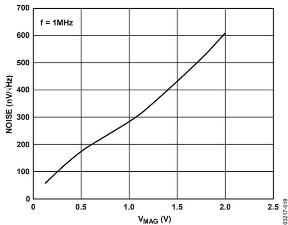
Figure 18. Output Referred Noise vs.  $V_{MAG}$ ,  $V_{DBS} = 0.75$  V
