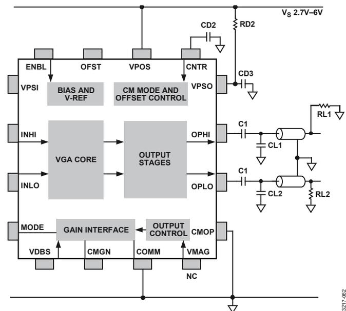
Figure 61. Driving Dual Cables with Grounded Loads
