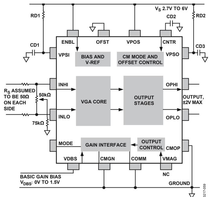
Figure 58. Input Offset Nulling in a DC-Coupled System
