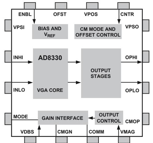
Figure 46. Block Schematic
