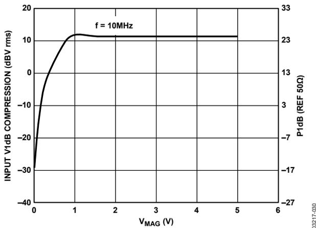
Figure 29. Output V1dB Compression vs. V<sub>MAG</sub>
