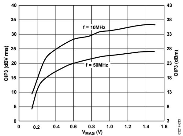
Figure 32. OIP3 vs. V<sub>MAG</sub>
