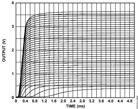
Figure 68. Time Domain Response of RMS Voltmeter (Simulation)
