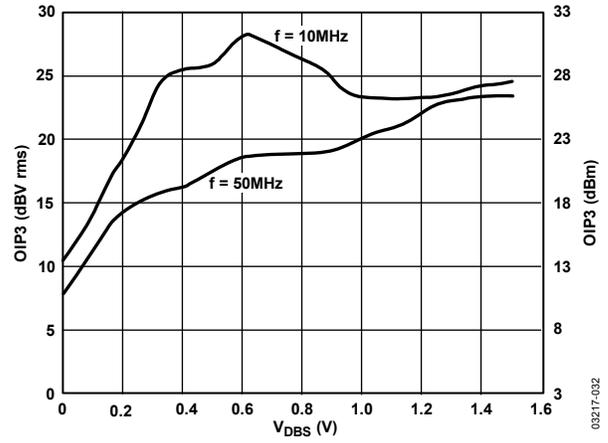
Figure 31. OIP3 vs. V<sub>DBS</sub>
