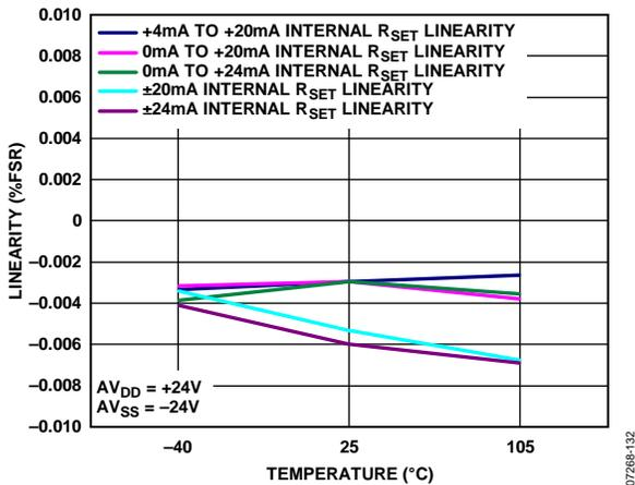
Figure 32. INL vs. Temperature, Internal R<sub>SET</sub> Sense Resistor
