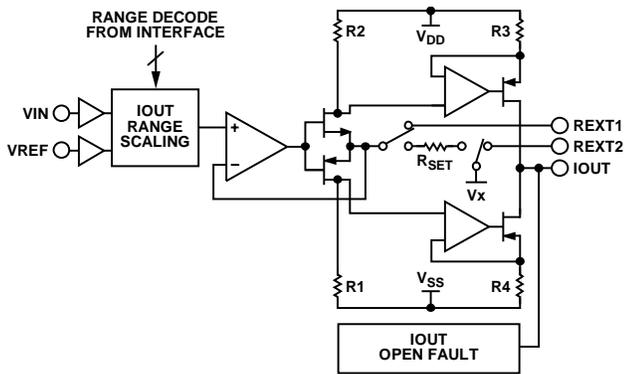
Figure 53. Current Output Configuration
