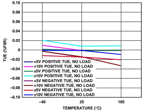
Figure 8. Total Unadjusted Error (TUE) vs. Temperature
