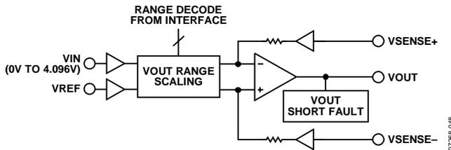
Figure 54. Voltage Output
