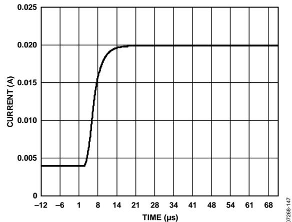
Figure 47. 4 mA to 20 mA Output Current Step
