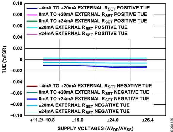
Figure 30. Total Unadjusted Error (TUE), Current Mode, External R<sub>SET</sub> Sense Resistor
