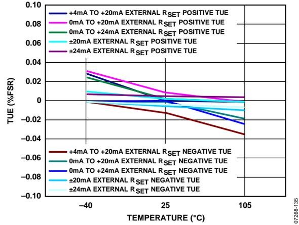
Figure 35. Total Unadjusted Error (TUE) vs. Temperature, External R<sub>SET</sub> Sense Resistor
