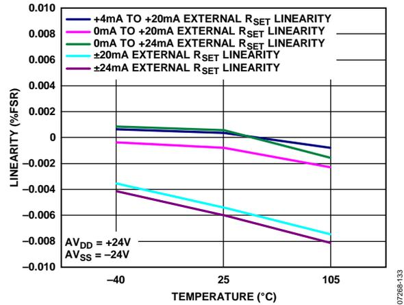
Figure 33. INL vs. Temperature, External R<sub>SET</sub> Sense Resistor
