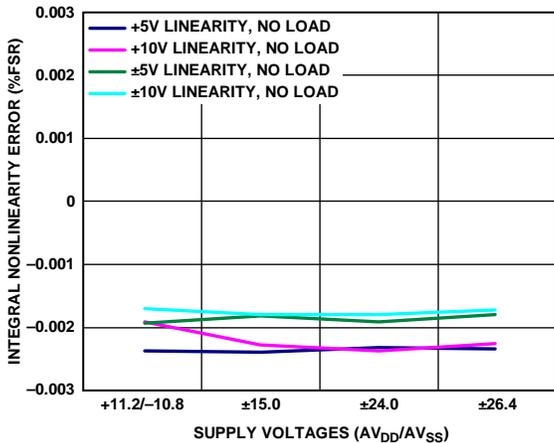
Figure 13. Integral Nonlinearity Error vs. Supply Voltage
