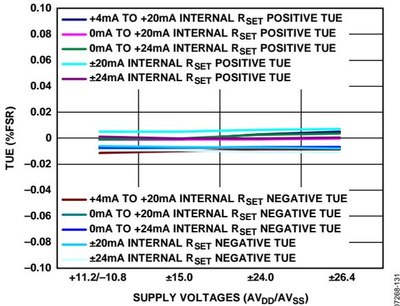
Figure 31. Total Unadjusted Error (TUE), Current Mode, Internal R<sub>SET</sub> Sense Resistor
