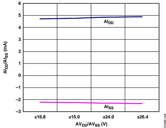
Figure 49.  $A_{IDD}/A_{ISSL}$  vs.  $A_{VDD}/A_{VSS}$ ,  $V_{OUT} = 0$  V
