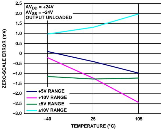
Figure 12. Zero-Scale Error (Offset Error) vs. Temperature
