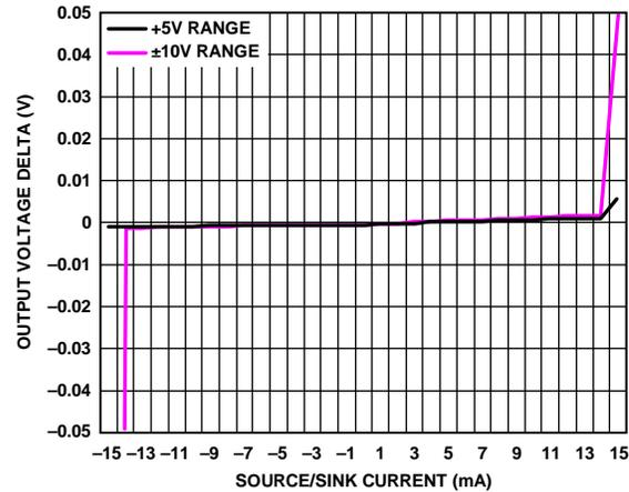
Figure 16. Source and Sink Capability of Output Amplifier
