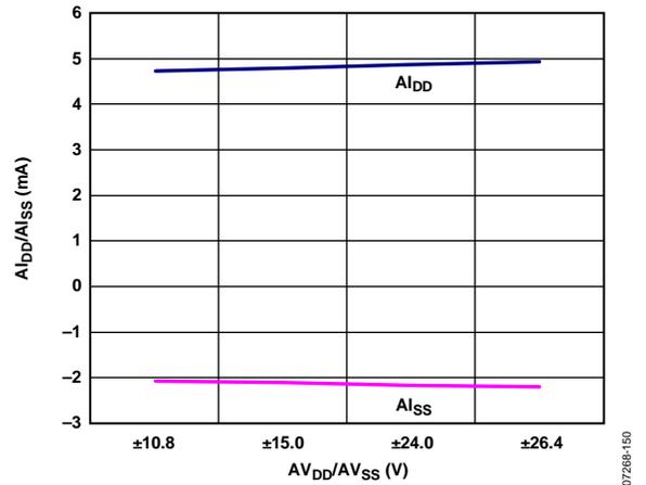
Figure 50.  $A_{IDD}/A_{ISSL}$  vs.  $A_{VDD}/A_{VSS}$ ,  $I_{OUT} = 0$  mA
