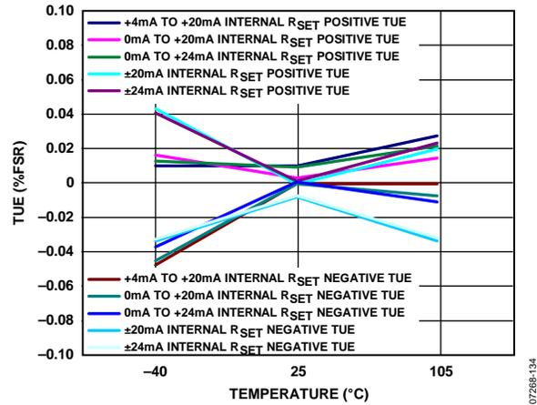
Figure 34. Total Unadjusted Error (TUE) vs. Temperature, Internal R<sub>SET</sub> Sense Resistor
